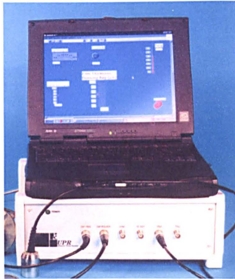
Figure 5.01. NDT Solutions Ltd UPR (with Laptop on top).
