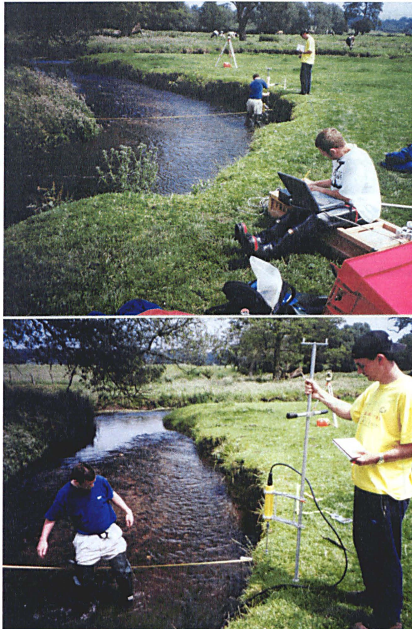
Figure 5.5: Positioning and Field methods. Total station (background) is used survey the bend morphology and position the ADV wading rod (foreground) into the same co-ordinate system. ADV data is downloaded onto a laptop.
