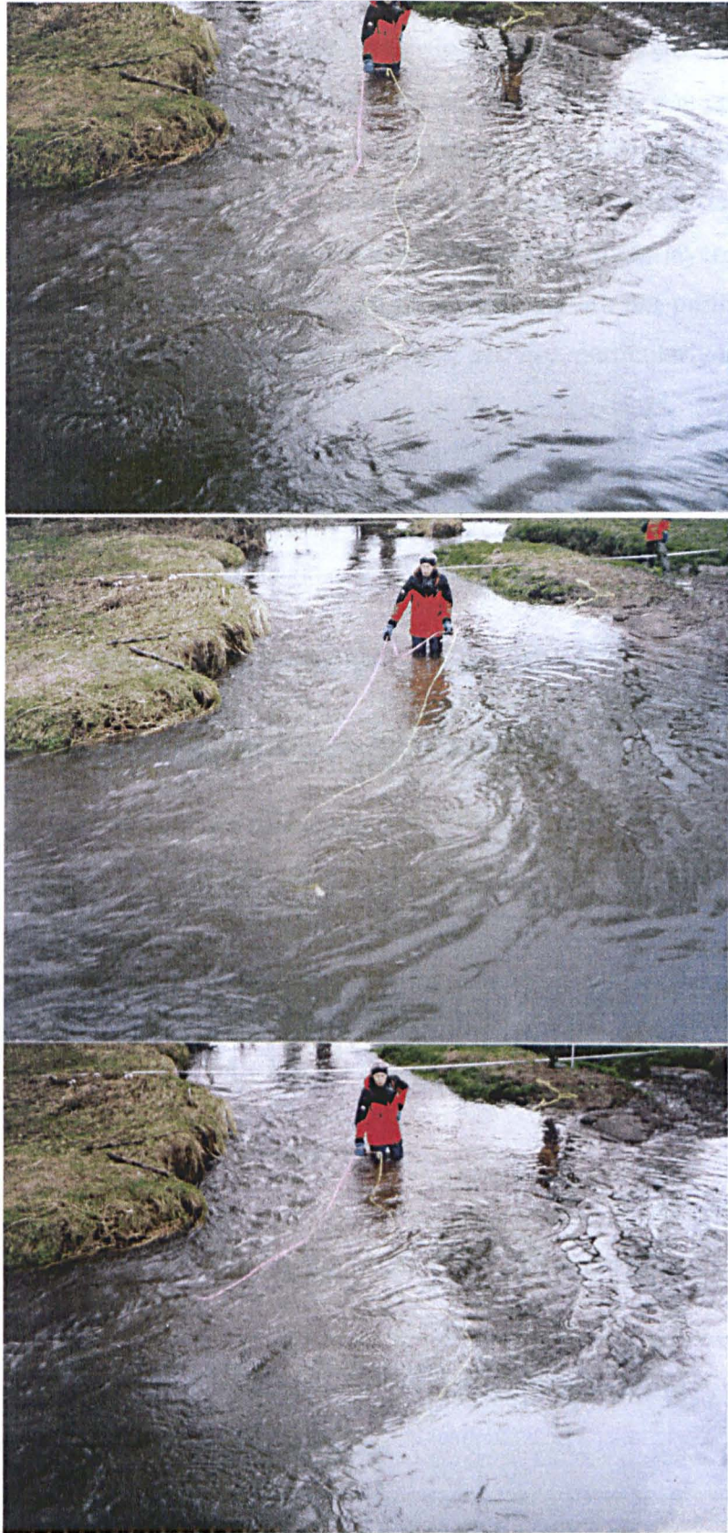
Figure 6.2: Sequential photographs of ribbons within the shear layer demonstrating large-scale coherent flow structures along the shear layer in bend 25 (looking upstream).
