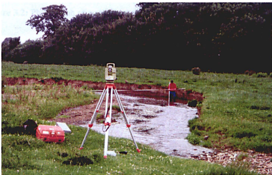
Figure 3.1: Photograph of methods used in surveying the channel cross sections with tapes placed across the channel.
