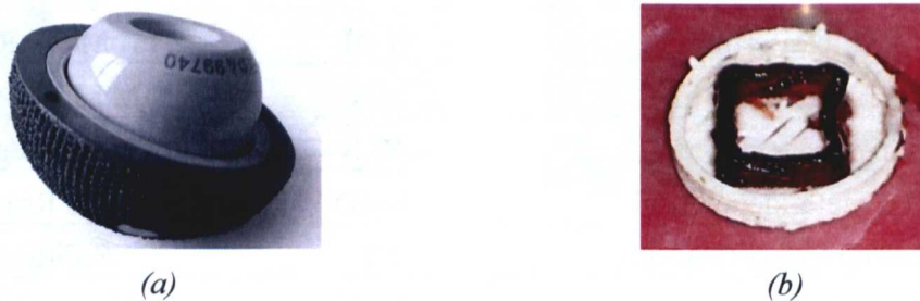
Figure 2.15 : Examples of graded ALM structures (a) Ti-6Al-4V acetabular cup graded by changing structure from fully dense to a porous outer mesh [43] and (b) a cheese and jam hors d'oeuvre showing how multiple materials can be used to grade structures and the potential for multiple materials per layer in ALM [44].
