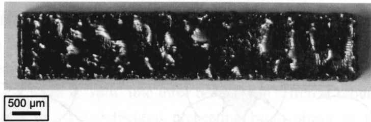
Figure 6.2 : Top surface of a Ti-6Al-4V-0.02B sample produced in the Arcam S12 with undulating surface on the surface.
