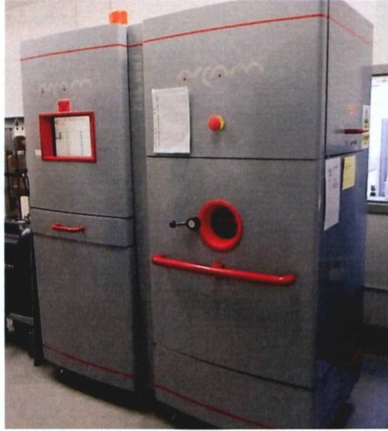
Figure 3.5 : Exterior of the Arcam S12. The left-hand unit houses the touch screen, computer and control/power units. The right-hand unit houses the build chamber and the electron gun.
