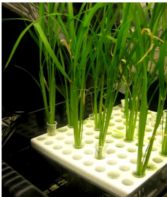
Figure 2.1. Hydroponic system for growing rice seedlings. Note that black plastic covering to prevent algal growth is not shown. Figure taken from Narawatthana 2013 (Thesis).
