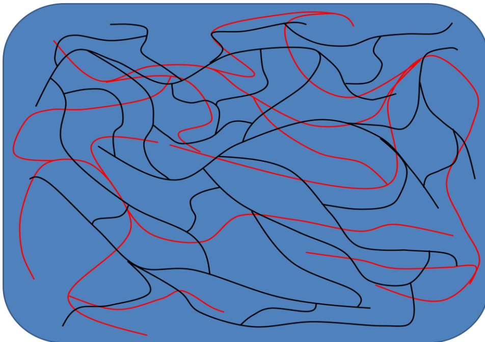
Figure 1.17 – A schematic diagram showing the structure of an interpenetrating polymer network produced by simultaneous or sequential polymerisations.
