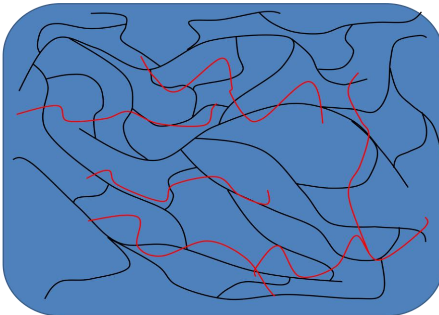
Figure 1.20 - A schematic diagram showing the structure of a semi-IPN with embedded linear polymer
