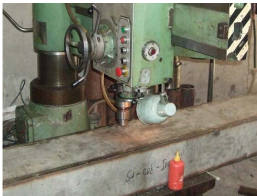
(a) Drilling process
