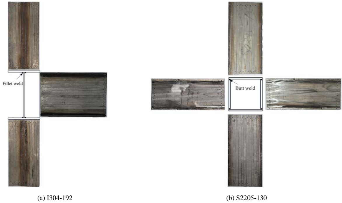
Fig. 7. Sliced residual stress test pieces
