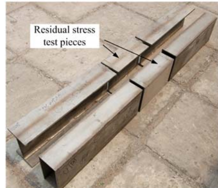
Fig. 6. Extraction of the test pieces
