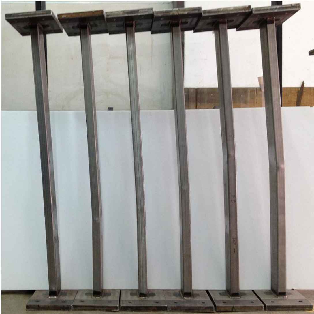
Fig. 12. Experimental failure modes for RHS 100×40×2-MI-1250 specimens (from left to right, the end moment ratios \psi are equal to -0.71, -0.35, 0.07, 0.31, 0.75 and 1.00).
