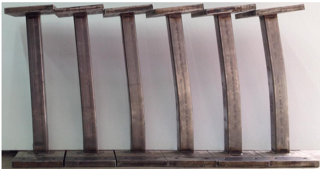
Fig. 13. Experimental failure modes for SHS 60×60×3-600 specimens (from left to right, the end moment ratios \psi are equal to -0.66, -0.26, -0.03, 0.31, 0.75 and 1.00).
