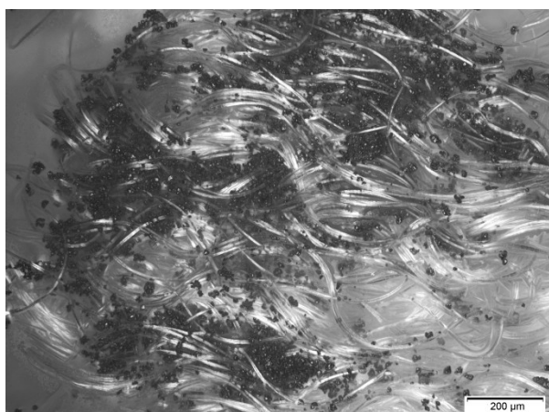
Figure 6.12 Epi-brightfield optical micrograph of the microfibre cloth after cleaning the soiled polystyrene substrate with isopropyl alcohol (scale bar = 200 \mu\text{m} ).
