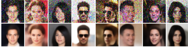
Figure 2: Reconstructions of faces from a DVAE trained with additive Gaussian noise: Q(\tilde{X}|X) = \mathcal{N}(X, 0.25\mathbf{I}) . The model successfully recovers much of the detail from the noise-corrupted images.
