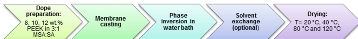
Figure 7.1 – Schematic representation of the steps involved in the PEEK membrane preparation.
