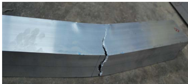
Fig. 6: Failure of test specimen by material tensile (N70×120×10.5B5III)
