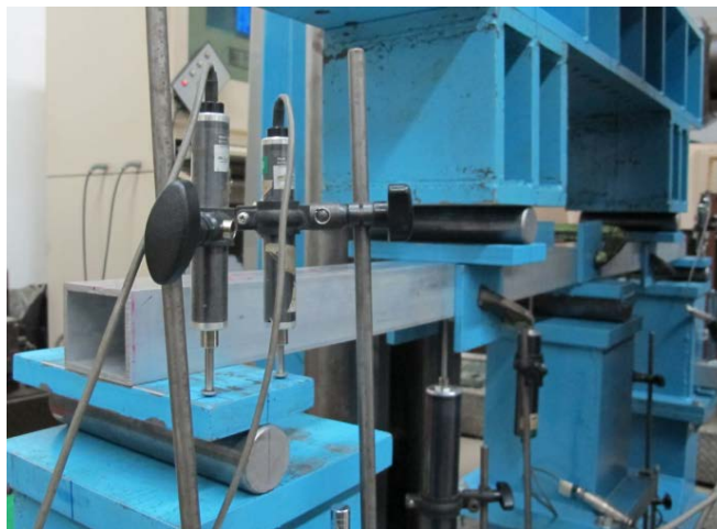
Fig. 4. Experimental setup for five-point bending test
