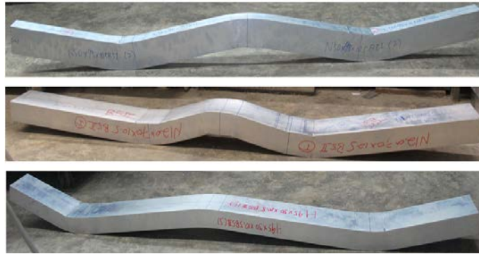
Fig. 5: Deformed five-point bending test specimens (N50×95×10.5B5I, N120×70×10.5B5II and H95×50×10.5B5III)
