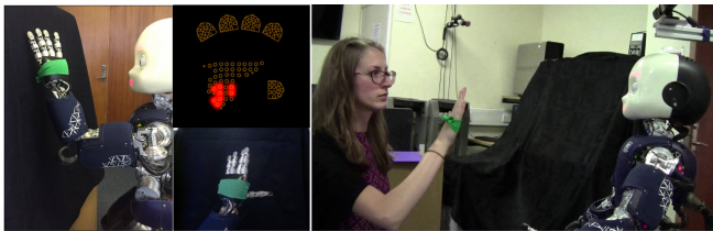
Fig. 2. (Left) iCub faces a surface and performs movements in order to touch it, with the palm touch sensor being activated during touch events (centre top) and the view from the robot's left eye camera (centre bottom). (Right) iCub learns to imitate a circular trajectory demonstrated by a human.
