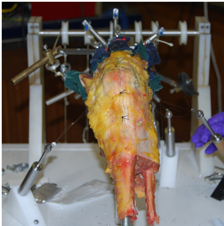
Figure 6.8 A cadaver knee mounted in the knee extension rig.
