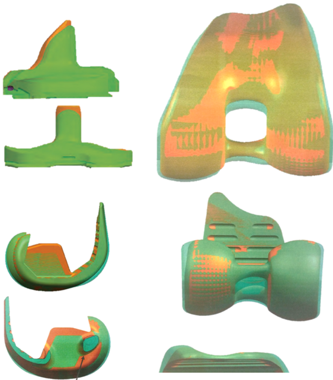
Figure 6.2 Comparison of the Journey and Journey II designs. Green = Journey. Orange = Journey II. A: higher, more anterior tibial spine and greater slope on the lateral compartment. B: bigger box, anterior cam moved anteriorly and posterior cam moved superiorly. C: narrower ML width. D: smaller anterior flange and narrower condyles.
