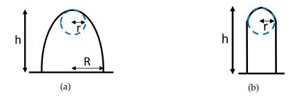
Figure 6.31: Parameters for (a) spheroid and (b) cylindrical protrusions from wire surfaces.
