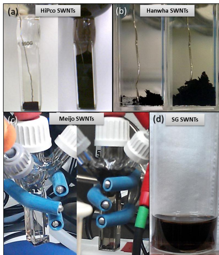
Fig. III-17 Photographs of the electrochemical dissolution of various commercial SWNTs synthesised via different processes. All SWNTs were dissolved at -2.3 V vs. Ag/Ag + for different lengths of time. (a) Raw HiPco SWNTs, (b) Hanwha SWNTs (ARC), (c) Meijo SWNTs (ARC), and (d) SG SWNTs (water-assisted CVD).
