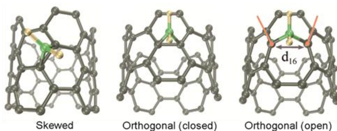
Fig. I-12 Three possible configurations for a carbene group ( \text{CH}_2 ) on a (5,5) armchair SWNT: skewed, orthogonal with an intact (“closed”) side-wall bond, and orthogonal with a broken (“open”) sidewall bond. The latter structure maintains the sp^2 hybridisation of the two side-wall C atoms, reducing the effect of functionalisation on the electronic properties of the SWNT. Reproduced from ref. 126.
