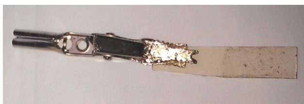
Fig. IV-5 Photograph showing electrodeposition of HiPco SWNTs on an ITO electrode at +0.5 V, 24 h. Deposition is highly aggregated due to the extreme change in oxidation potential.
