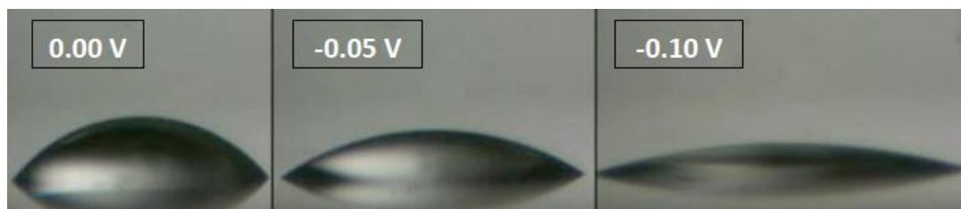
Figure 5 |[Taken from Cousens 9 ] A recreation of Frumkin's experiment from 1932. A 1,2-dichloroethane droplet sits on a mercury electrode surround by 0.1 \text{ mol dm}^{-3} LiCl solution. Potentials are versus an Ag/AgCl reference electrode.
