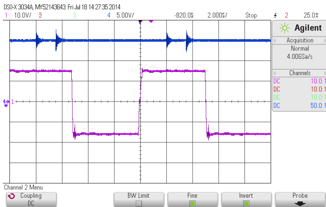
Fig. 20. The input voltage (bottom) of the primary coil and the output voltage (top) of the system at the initial point when R_L = 50 \Omega .
