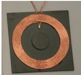
Fig. 7. The coil of a practical WPT system.
