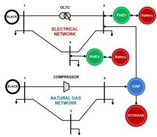
Fig. 1. Energy networks coupled through new technologies, such as PHEV and CHP, might increase the efficiency in power provision.
