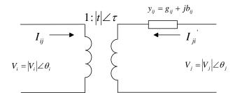
Fig. 2. Representation of an on-load tap-changer transformer (OLTC).
