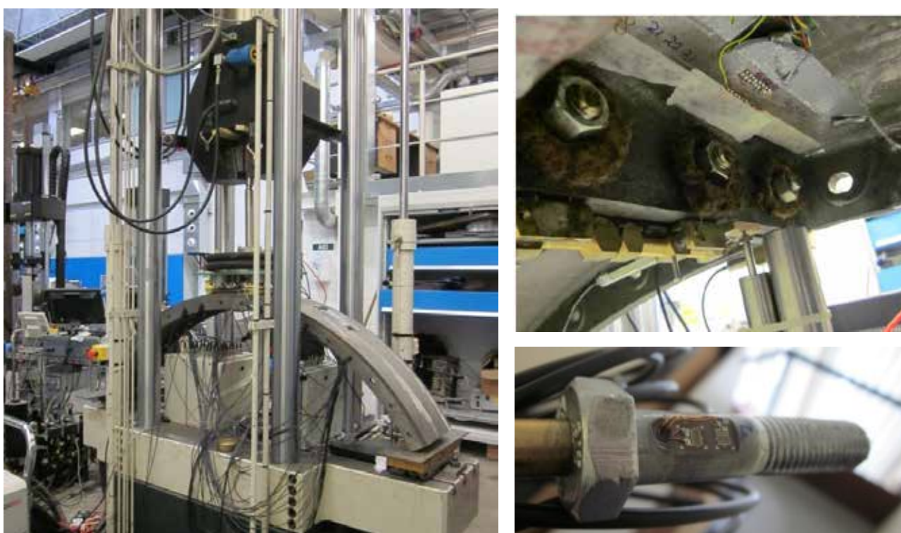
Figure 4: Two-segment test set-up and details of instrumentation across joint and on bolts
