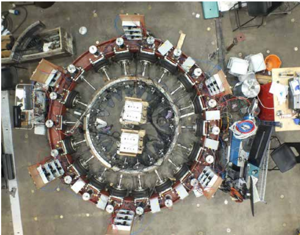
Figure 5: Aerial view of half-scale full-ring test set-up (red outer ring provides load reaction for actuators)
