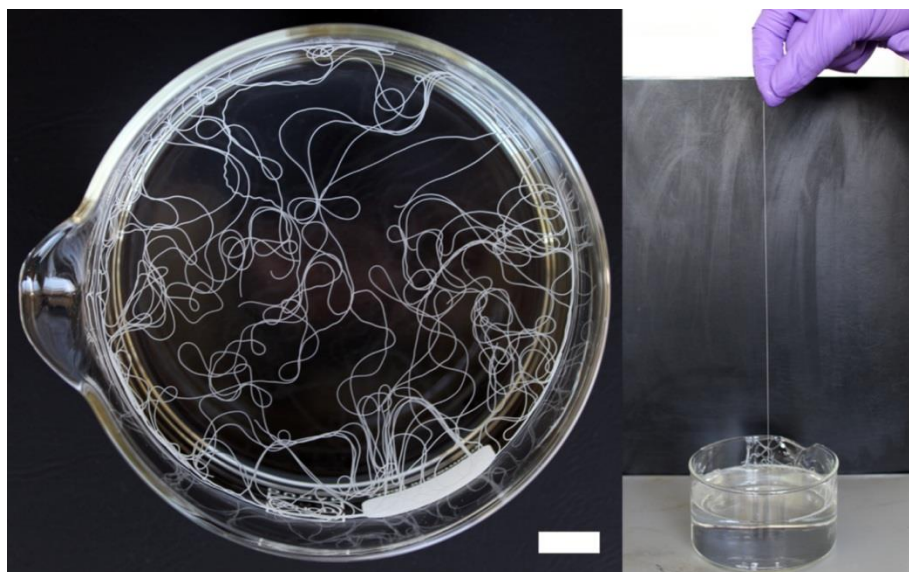
Figure 3.14. HIPE fiber fabricated with acidic water as sheath fluid. Scale bar represents 1 cm. Several fragmented fibers arise from blockage of capillaries and viscosity mismatch of the concentrated emulsion and sheath fluid.
