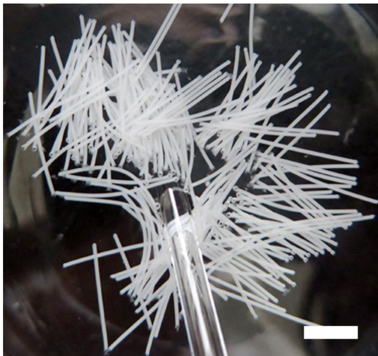
Figure 3.17. Photograph of HIPE fibers with uniform length. The HIPE fibers with uniform length were fabricated by utilizing air bubbles as a cutting mechanism. Scale bar represents 0.5 cm.
