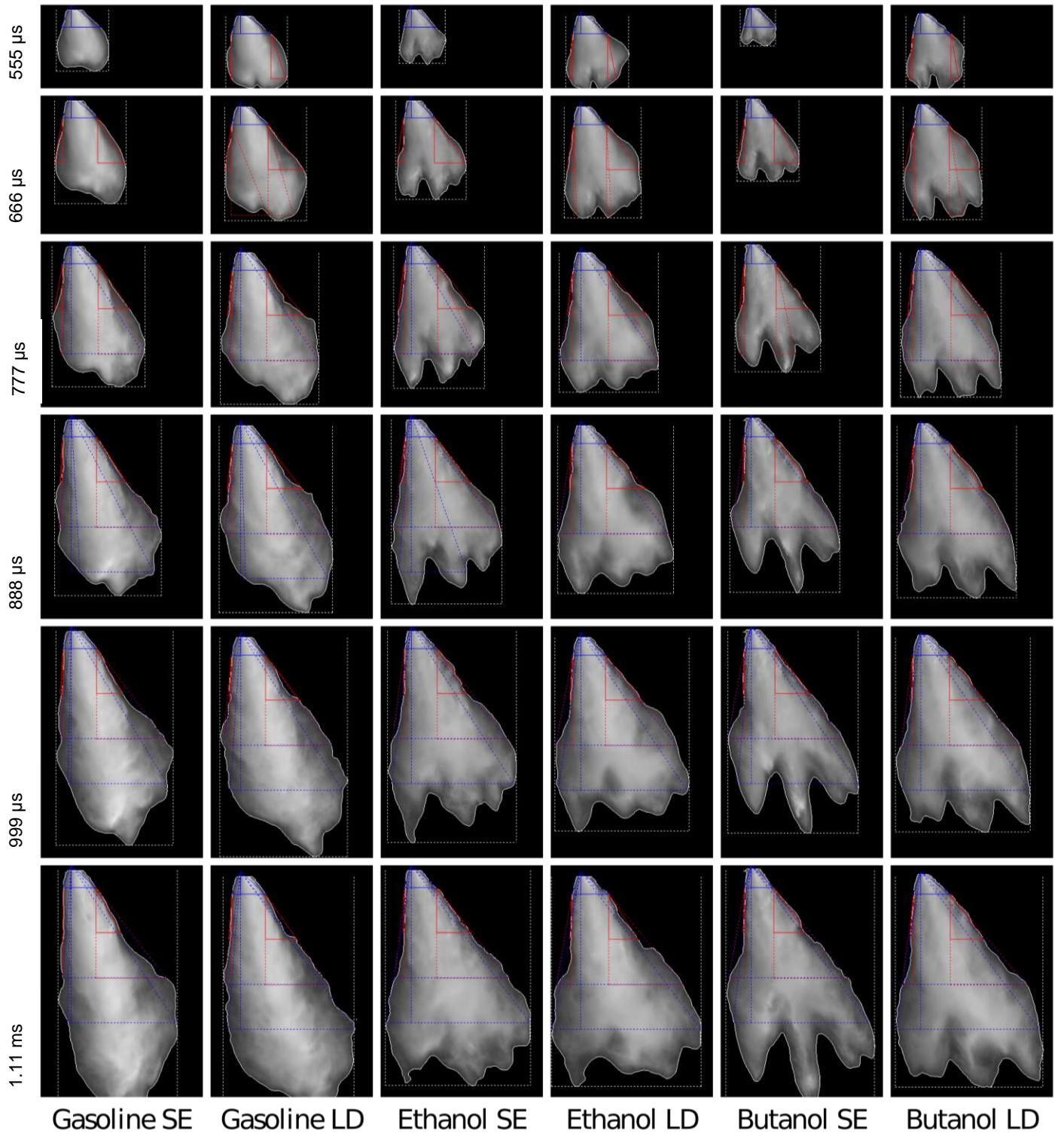
Figure 30. Spray imaging at 80 °C injector temperature, 1 bar air pressure.
