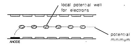
Figure 44: Pockets of undepleted silicon within the detector
