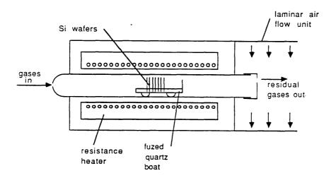
Figure 19: The oxidation furnace
