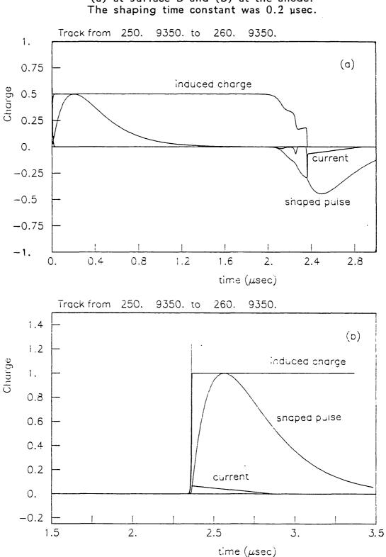
Figure 61: Signals induced by charges for 7.0 mm drift distance Induced charge, current and shaped output pulse (a) at surface B and (b) at the anode. The shaping time constant was 0.2 user
