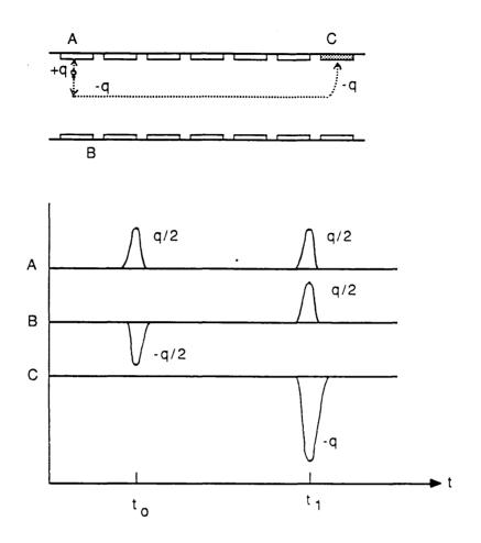
Figure 59: Development of signals due to charge deposited in the SDC
