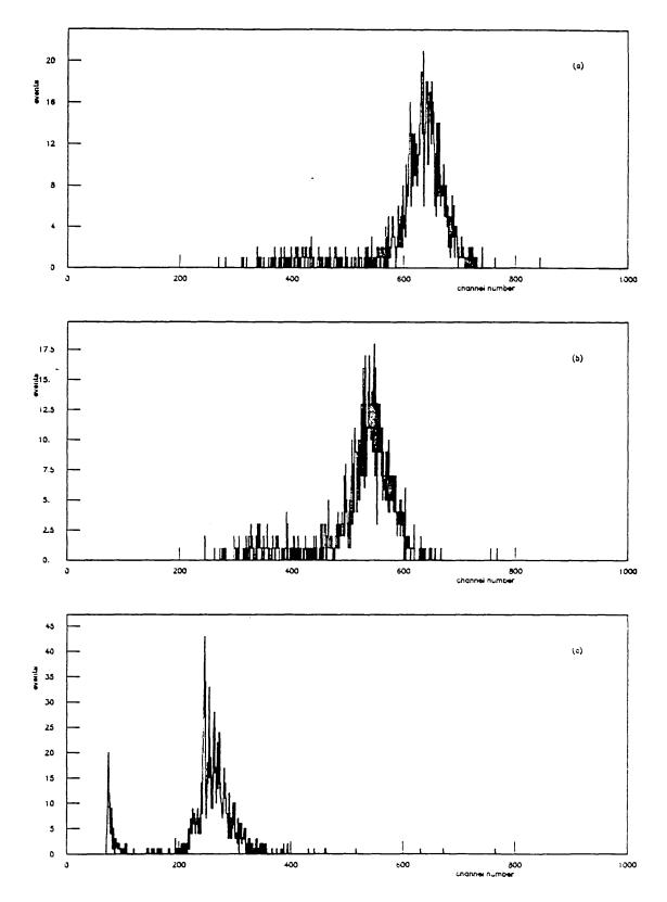
Figure 52: Time spectra of pulses in the SDC for drift distances of (a) 4.5 mm, (b) 3.5 mm and (c) 0.5 mm.
