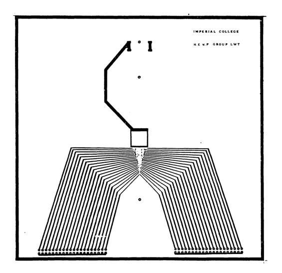
Figure 29: The fan out printed circuit board
