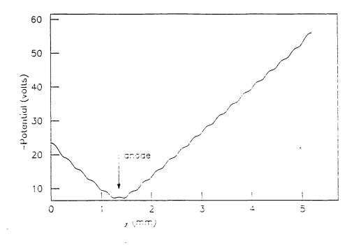
Figure 43: Undulations in the potential minimum at the centre of a silicon drift chamber.
