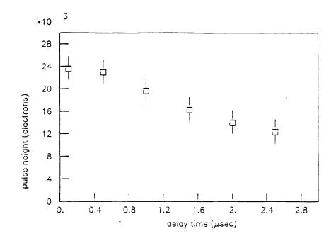
Figure 42: Pulse height as a function of time delay
