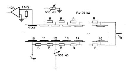
Figure 49: Biasing arrangement for observation of drift action
