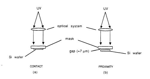
Figure 22: Optical lithographic exposure techniques (a) Contact printing. (b) Proximity printing.
