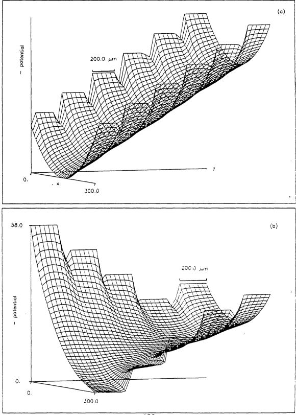
Figure 56: Calculated potential distribution in the SDC (a) in the drift region and (b) in a region close to the anode.
