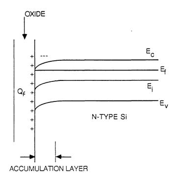
Figure 67: Band-bending at the surface of an n-type semiconductor due to the presence of oxide fixed charge .
