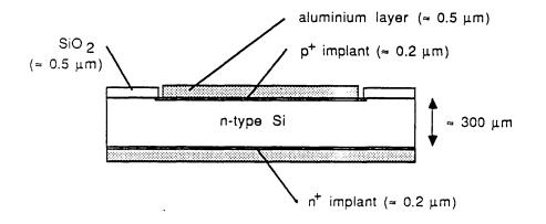
Figure 1: Cross-section through a typical ion implanted detector
