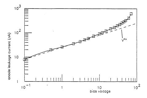
Figure 48: Anode leakage current vs. bias voltage
