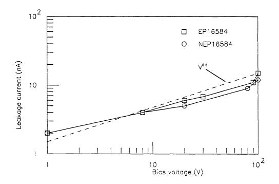
Figure 8: Leakage currents plotted against bias voltage for detectors EP-16584 and NEP-16584.
