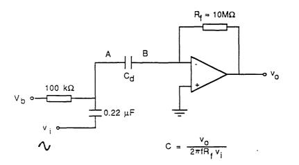
Figure 33: Circuit used for capacitance measurements
