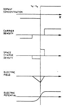
Figure 5: Properties of the step junction model (a) Dopant concentration, (b) carrier density, (c) space charge density, (d) electric field and (e) electric potential.
