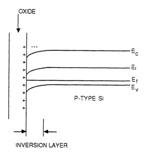
Figure 7: Band-bending due to oxide fixed charge at the surface of a p-type semiconductor.
