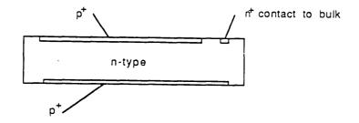
Figure 15: Practical means of contacting the n-type silicon via an  $n^+$  implant at one side of the detector.
