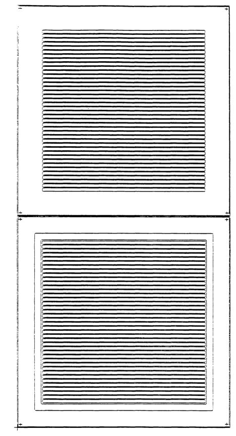
Figure 25: Magnified diagram of a pair of SDCs The bottom SDC has a guard ring incorporated in the design.
