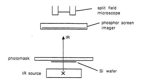
Figure 28: The infra-red alignment system
