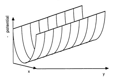
Figure 16: Potential of a fully depleted silicon wafer when an additional constant field along the y-axis is applied.
