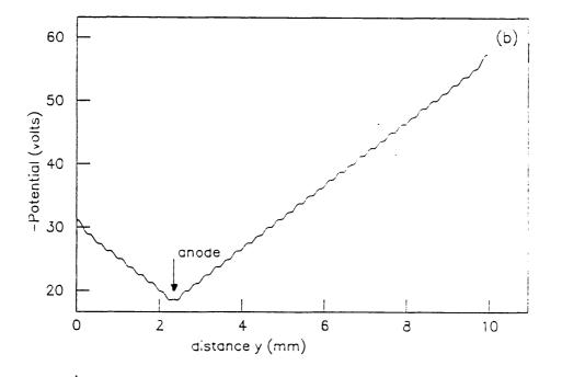
Figure 63: Variation of the potential minimum (a) Potential distribution in the SDC in a region close to the anode. (b) Variation of the potential along the centre of the detector (x = d/2). The drift field was 50 V/cm.
