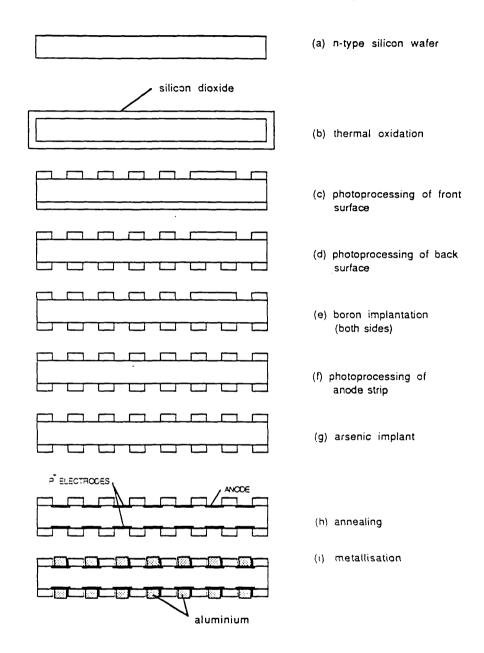
Figure 26: Processing steps in the fabrication of the SDCs
