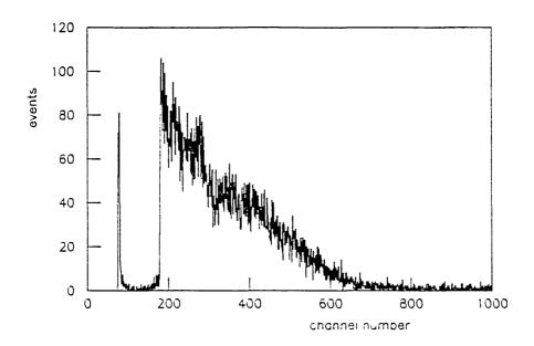
Figure 39: Time spectrum of signals in the SDC
