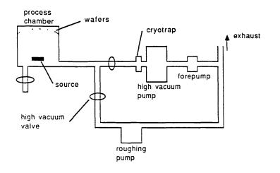
Figure 23: Schematic representation of the high vacuum chamber · used for the metallisation process.
