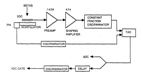
Figure 38: Electronics chain used for timing measurements
