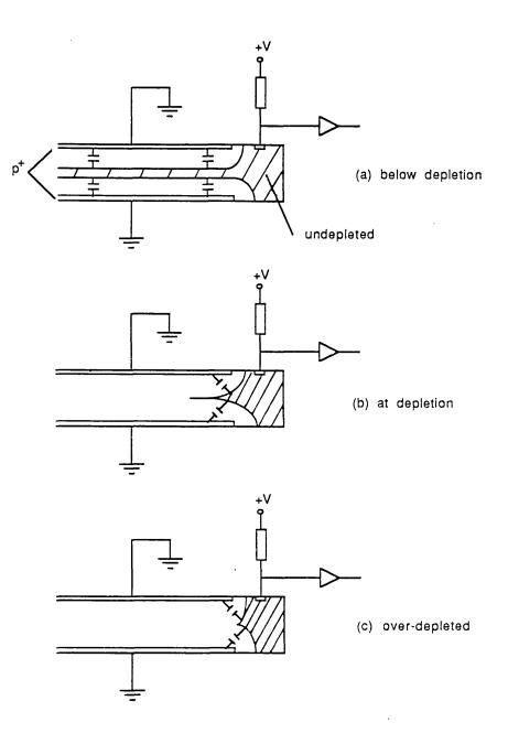
Figure 32: Capacitance between all p<sup>+</sup> electrodes and the anode
