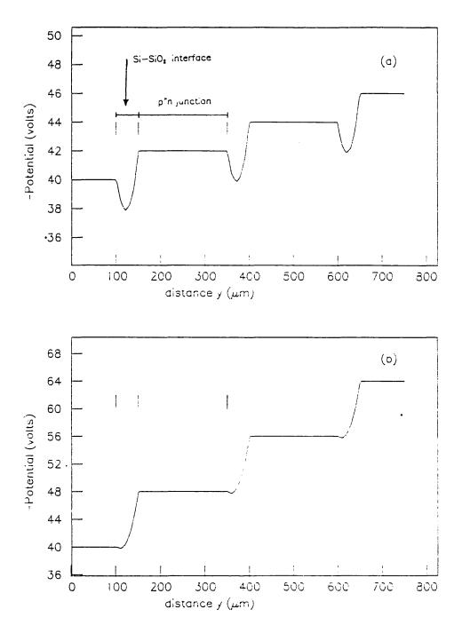
Figure 65: Potential distribution along the surface of the SDC with an applied voltage increment between adjacent strips of (a)  $\Delta V$  less than  $V_T$  and (b)  $\Delta V$  just less than  $V_T$ .
