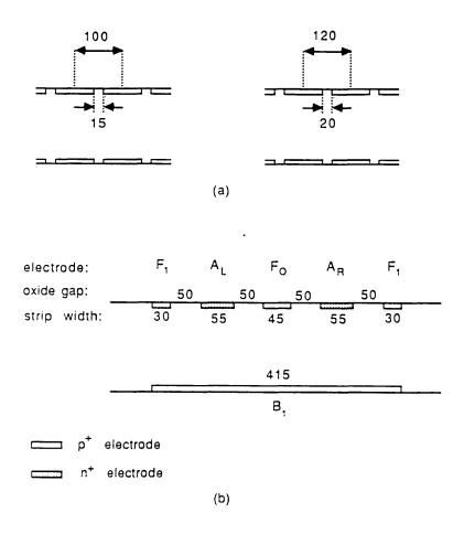
Figure 69: Cross-sectional view of the new SDC designs (a) in the drift region and (b) in the anode region.
