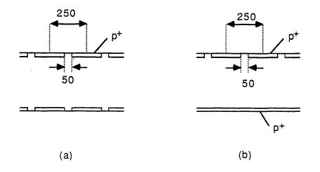
Figure 30: Cross-sections of the SDC designs (a) Standard design. (b) Single-area  $p^{+}$ electrode on one side.
