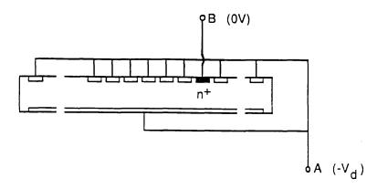
Figure 34: Biasing arrangement for the CV measurements
