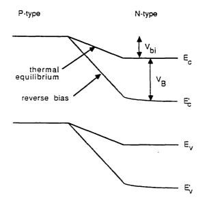
Figure 6: Energy level diagram for reverse bias at thermal equilibrium.
