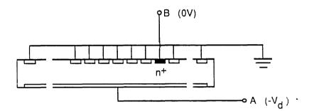
Figure 37: Biasing arrangement for CV measurement of figure 35(b)
