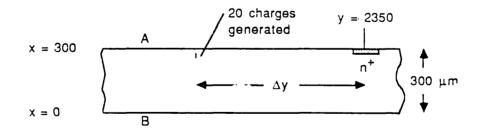
Figure 60: Generation of charge in the SDC for modelling the output signals.
