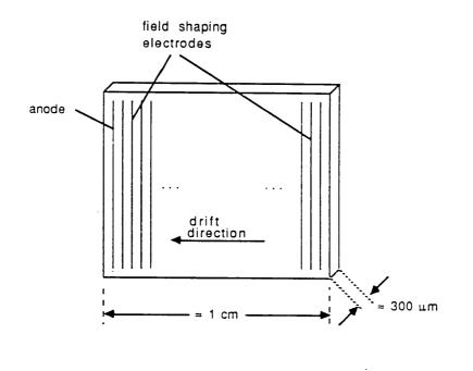
Figure 17: Practical realisation of a silicon drift chamber
