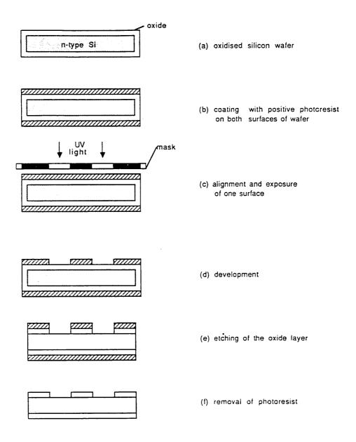
Figure 27: Basic steps in the photolitography for double-sided polished silicon.
