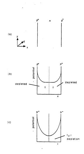
Figure 14: Depletion of a single n-type semiconductor with  $p^{+}$  junctions on both sides.
