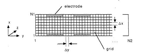
Figure 54: Schematic representation of a silicon drift chamber showing the grid lines used for the numerical solution to Poisson's equation.
