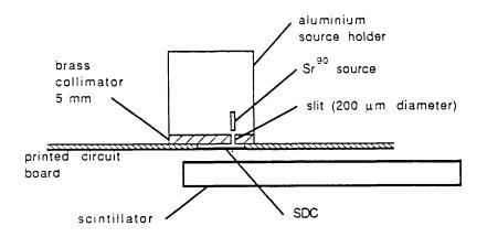
Figure 50: Experimental set up for observation of signals
