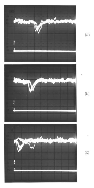
Figure 51: Waveforms at the output of the shaping amplifier for drift distances of (a) 4.5 mm, (b) 3.5 mm and (c) 0.5 mm. The scope was triggered on the scintillator pulse (lower trace). The timebase was 0.5 µsec/div and the voltage scale was 0.5 V/div on all traces.
