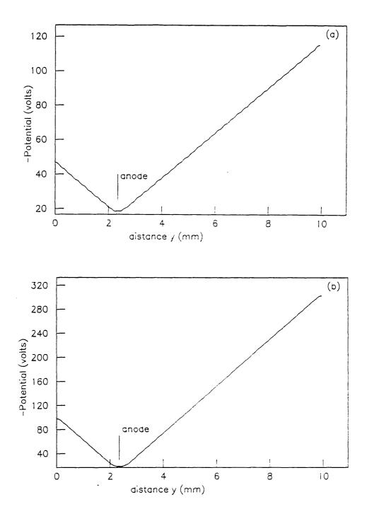
Figure 64: Variation of the potential along the centre of the SDC for drift fields of (a) 130 V/cm and (b) 390 V/cm.
