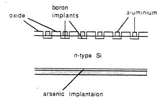
Figure 10: Cross-section through a microstrip detector
