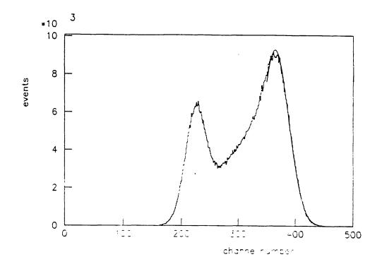
Figure 45:  $Am^{241}$  3 spectrum obtained with an SDC showing the 59.5 keV 3 line. Also plotted is the result of a Gaussian fit to the high energy part of the peak.
