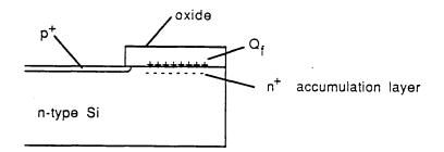
Figure 20: Effect of oxide fixed charge on a planar p<sup>+</sup>n detector
