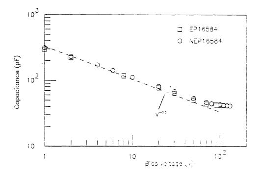
Figure 9: Capacitance characteristics of detectors EP-16584 and NEP-16584.
