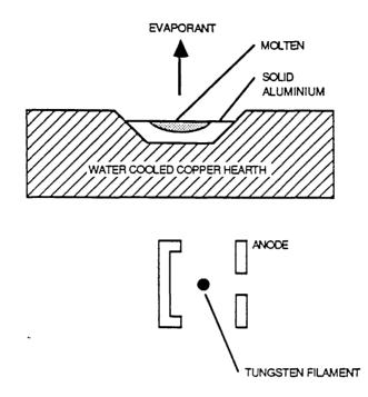
Figure 24: The electron beam evaporation system
