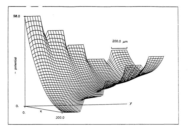
Figure 18: Potential within a silicon drift chamber in a region close to the anode.
