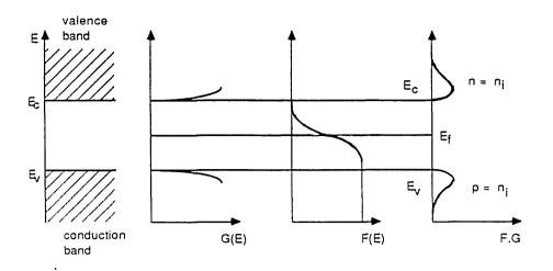
Figure 3: Intrinsic semiconductor at equilibrium Schematic band diagram, density of states, Fermi-Dirac distribution and carrier concentrations.
