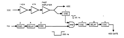
Figure 40: Electronics chain used for pulse height measurements
