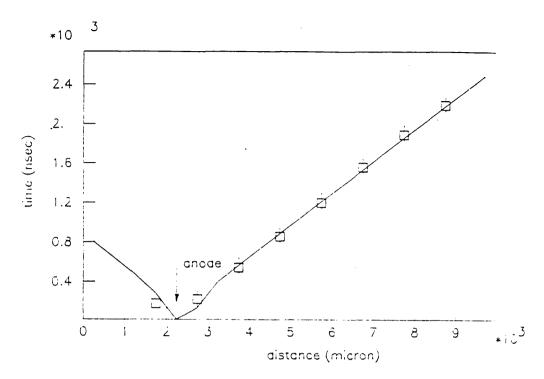
Figure 58: Simulated distance-time relationship for SDC (solid line). Also plotted are the experimental data points (squares).
