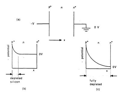
Figure 12: Depletion of a standard p n junction detector
