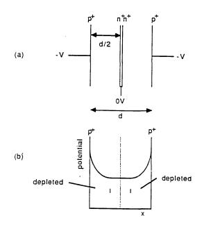
Figure 13: Two standard p<sup>\*</sup>n detectors in proximity (a) With n<sup>\*</sup> electrodes in contact. (b) Potential and depletion regions of the two detectors under reverse bias.
