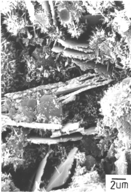
PLATE 5.2.14 Fracture surface of 2 days old Westbury blended cement
