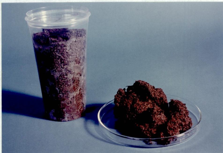
Plate 4.2. Artificial soil test: a one litre plastic flask containing 750 g hydrated artificial soil is shown together with a sample of the soil.
