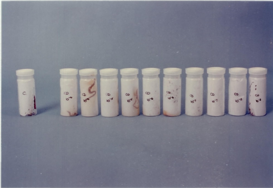
Plate 3.3. Filter paper contact test: the apparatus in use showing two replicates of each concentration of the test chemical and a control.
