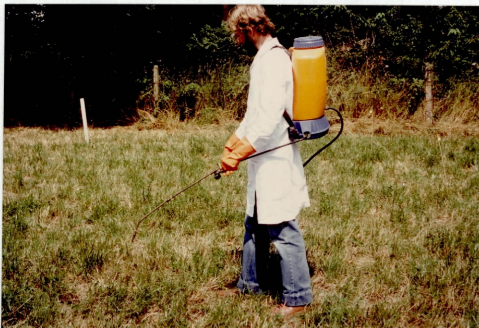
Plate 6.3. Application of the test chemical to the soil using a backpack sprayer.
