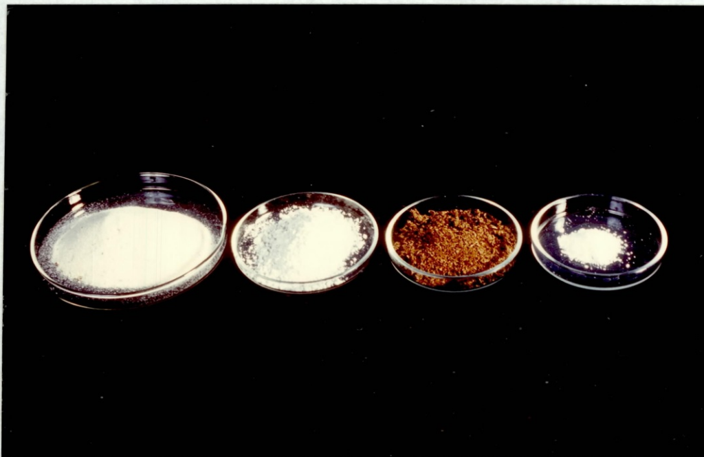
Plate 4.1. Artificial soil test: the components of the soil were (Left-Right) quartz sand, kaolinitic clay, airdried and milled peat and calcium carbonate.
