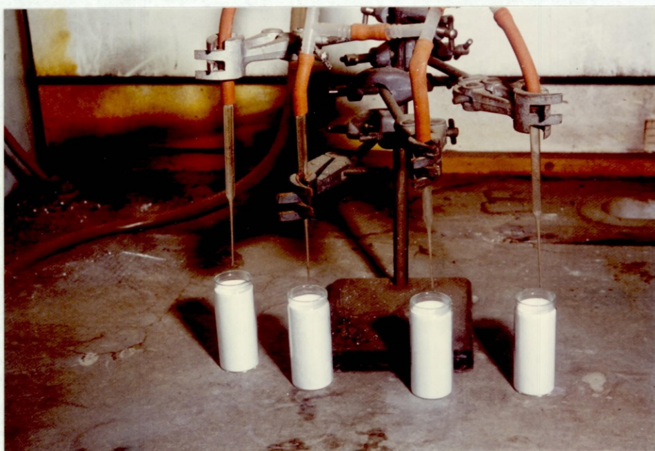
Plate 3.2. Filter paper contact test: evaporation of volatile organic solvent using compressed air.
