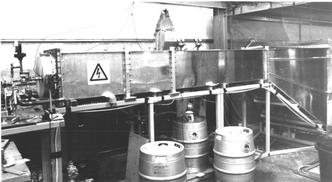
Fig. 6.2: Photograph of the new transmission line. Maximum current: 200kA.
