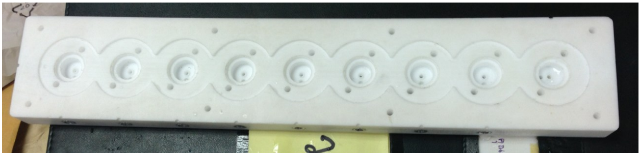
Fig 6.08 Part 1 (top) of solenoid valve manifold, containing vents and solenoid valve chambers.
