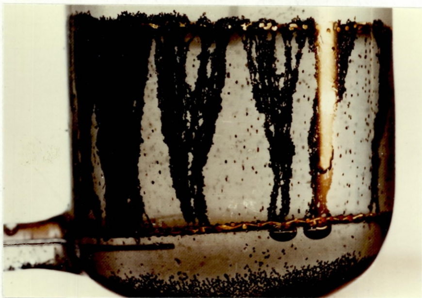
Plate 2.1.2. Chaining of Kimberlite Particles of size < 1 mm in kerosene. Quartz particles fall through without chaining.
