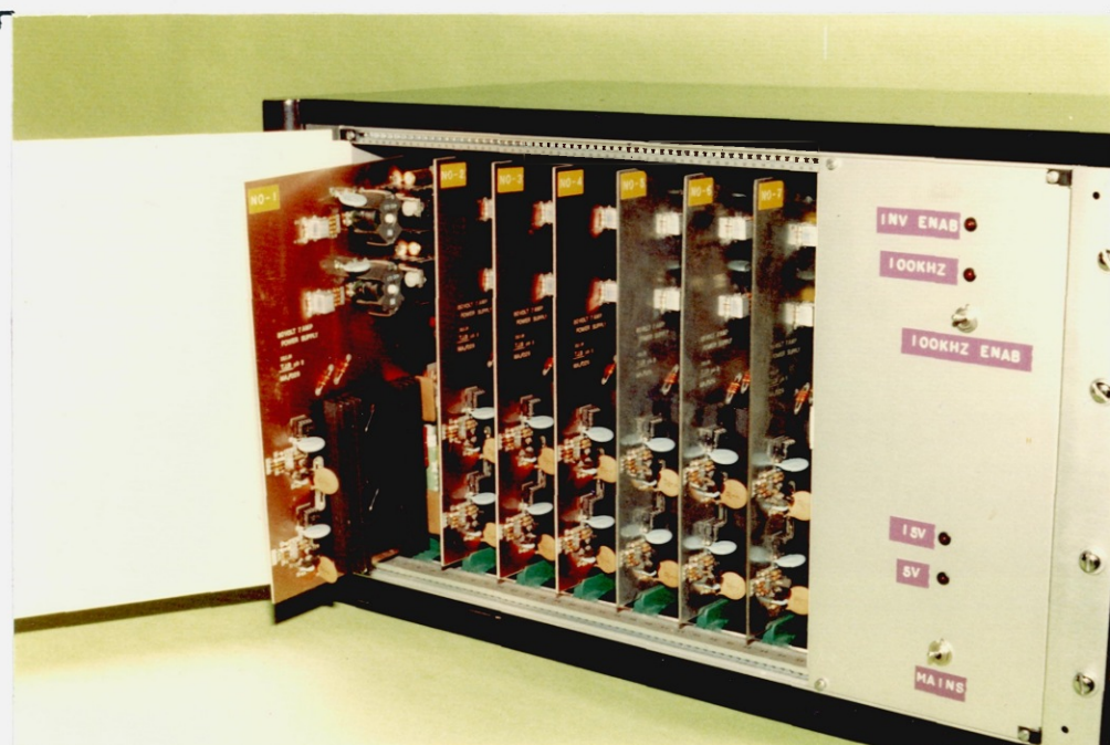
FIG. 5.27b. FRONT VIEW OF THE INVERTER UNIT SHOWING THE HEXFET CIRCUIT BOARDS, THE INDICATOR LEDES, AND CONTROL SWITCHES
