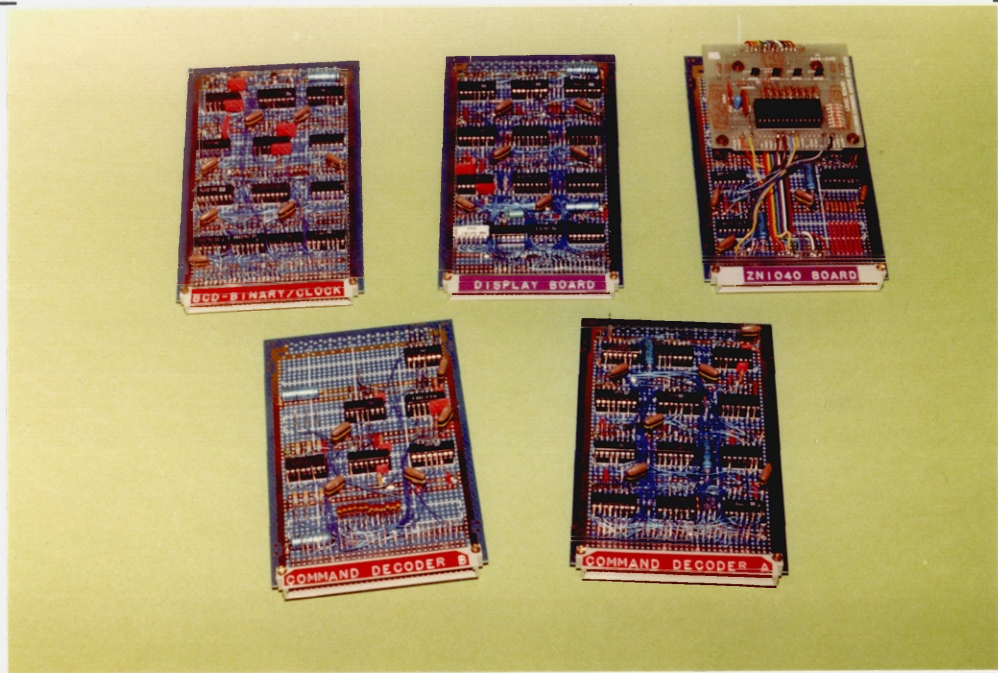
FIG. 7.15. PHOTOGRAPH OF THE AUXILIARY LOGIC UNIT KEYPAD-RELATED CIRCUIT BOARDS . THE DISPLAY BOARD AND THE ZN1040 BOARD FORM THE RECALLED DATA DISPLAY UNIT CIRCUIT.
