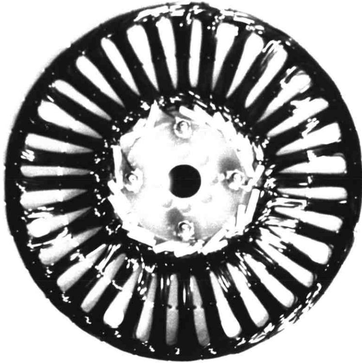
Fig. 5.3 - Wire-wound rotor coil assembled
