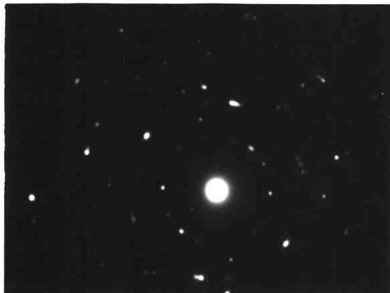
Fig. 3.15(b): Electron Diffraction Pattern of a CuInSe 2 Film after Anneal at 350°C for 30 hours
