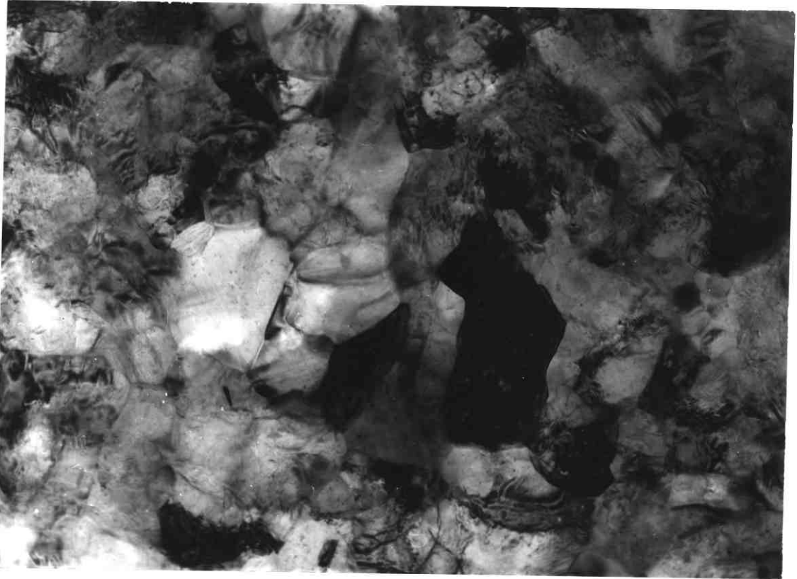
Fig. 3.13(a): Transmission Electron Micrograph of a CuInSe 2 Film after Anneal at 350°C for 3 hours (Mag = x 30,000)
