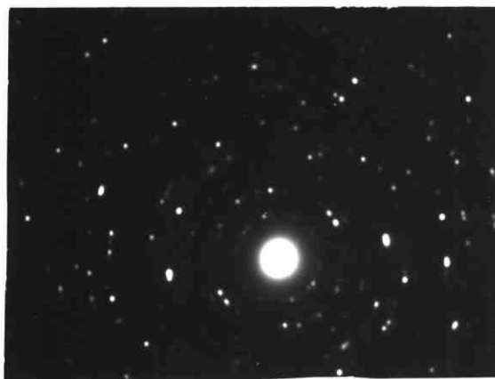
Fig. 3.13(b): Electron Diffraction Pattern of a CuInSe 2 Film after Anneal at 350°C for 3 hours
