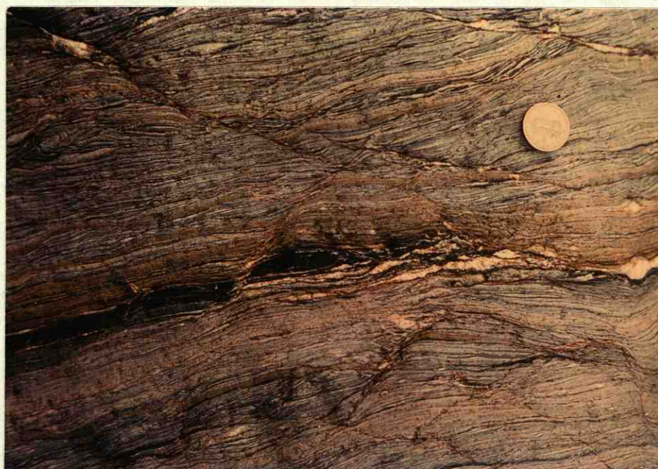
Fig. 3.4 A. Interlocking pinch-and-swell structures and incipient shears in metasediments - below Glarus Nappe, near Flimms, Swiss Alps, (after J. Cosgrove).
