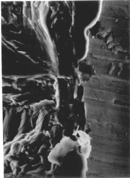
Fig. 4.40. Crack initiation at hole corner in deburred specimens
