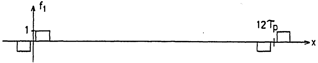
Fig. 3.16 Arbitrary MMF standing wave due to entry/exit region image currents.
