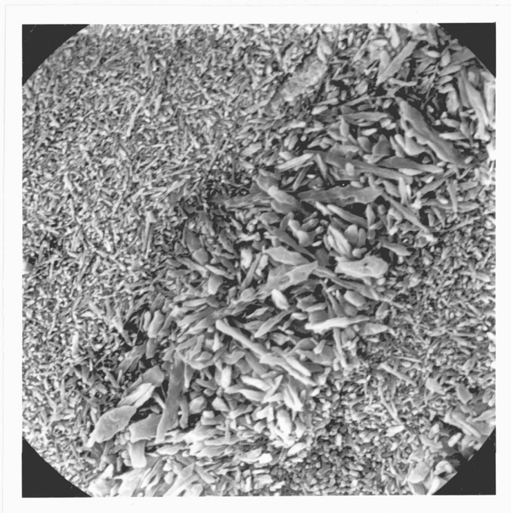
FIG.III.2. Electronmicrograph showing a lamella of randomly disposed aragonite crystals. Note 'platy' habit of crystals compared to the 'needles' of adjacent aragonite lamella. 1\text{cm} = 2.27\mu\text{m}
