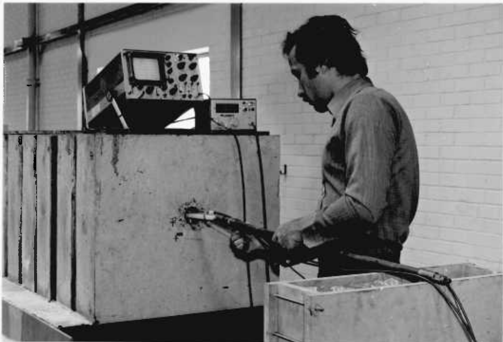
PLATE 6b Ultrasonic velocity logging of borehole at end B
