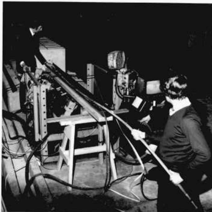
PLATE 5b Introducing camera into borehole at end A
