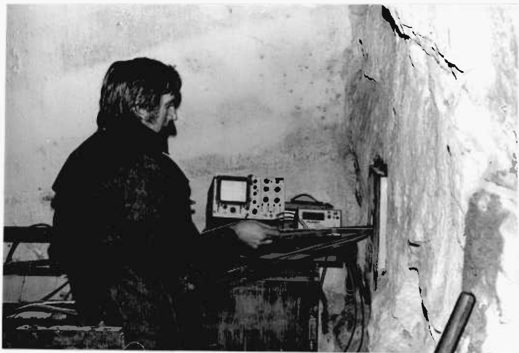
PLATE 10b Ultrasonic velocity logging of underground borehole at end A
