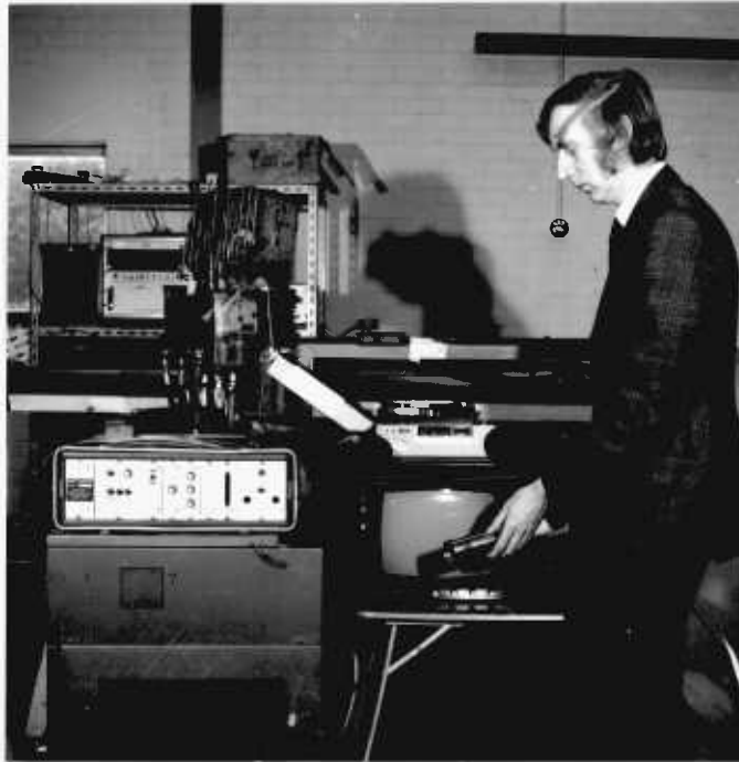
PLATE 4a Borehole television camera, television monitor, videotape recorder and control unit
