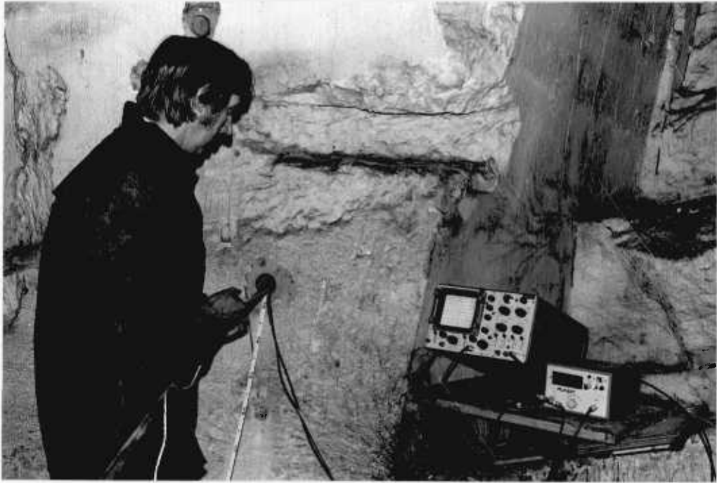
PLATE 10a Ultrasonic velocity logging of underground borehole at end B
