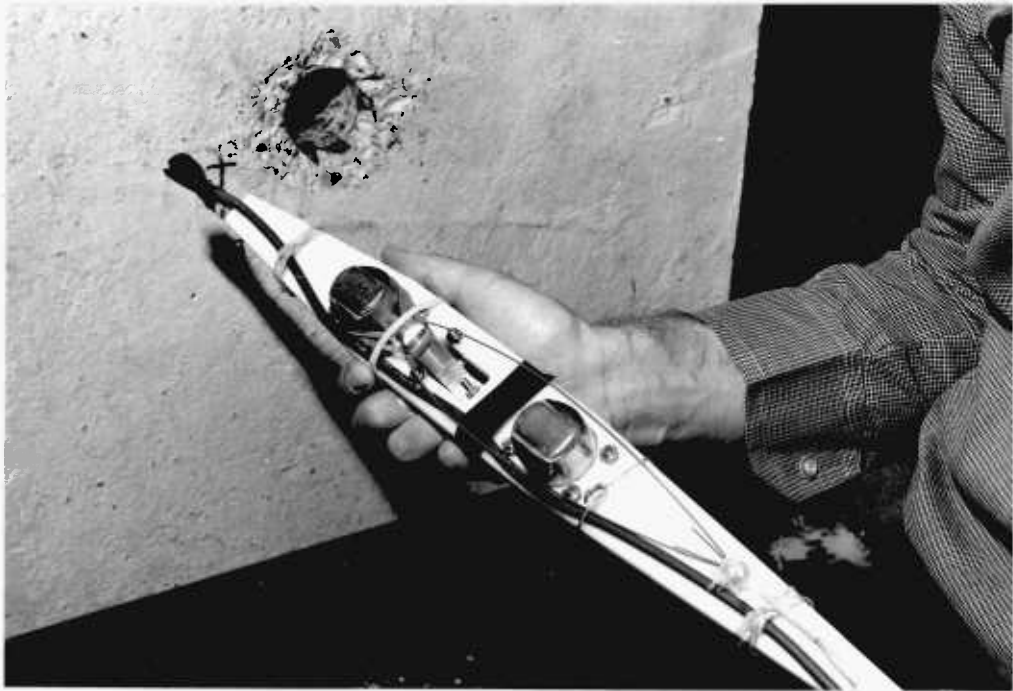
PLATE 6a Ultrasonic velocity tool
