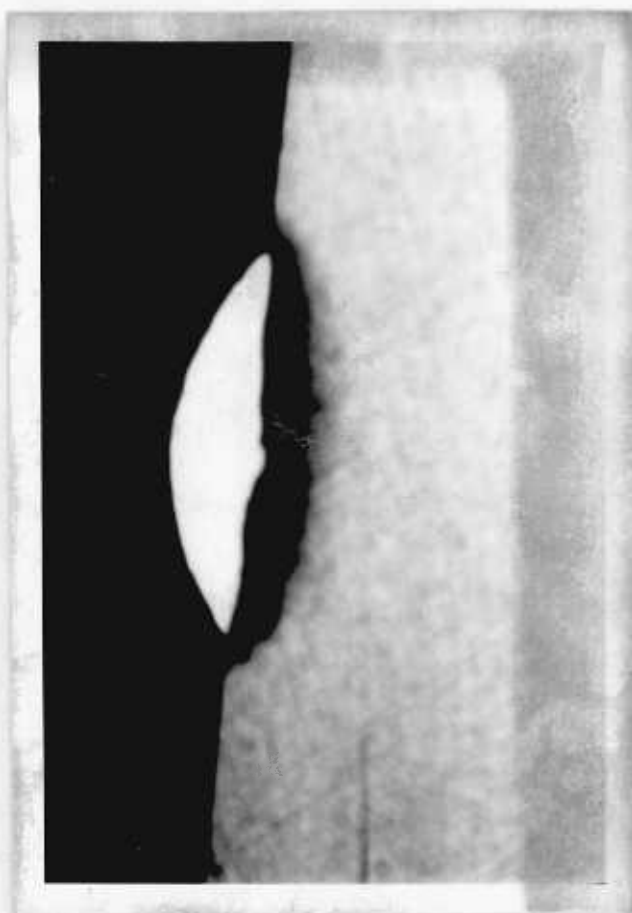
FIG 4.92 MICROHARDNESS AND MACROGRAPH SECTION VIEW THROUGH SURFACE CLADDING ETCHED 2% NITAL, X21, POWER=1 600 W BEAM DIAMETER=43 MM, SPEED=10 MM/S, POWDER THICKNESS = 0.50 MM.
