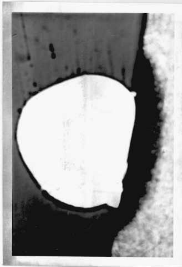
FIG. 4.94 MICROHARDNESS AND MACROGRAPH SECTION VIEW THROUGH SURFACE CLADDING ETCHED 2% NITAL, X21. POWER = 1 400 W BEAM DIAMETER = 0.7 MM, SPEED = 5 MM/S, POWDER THICKNESS = 1.00 MM.
