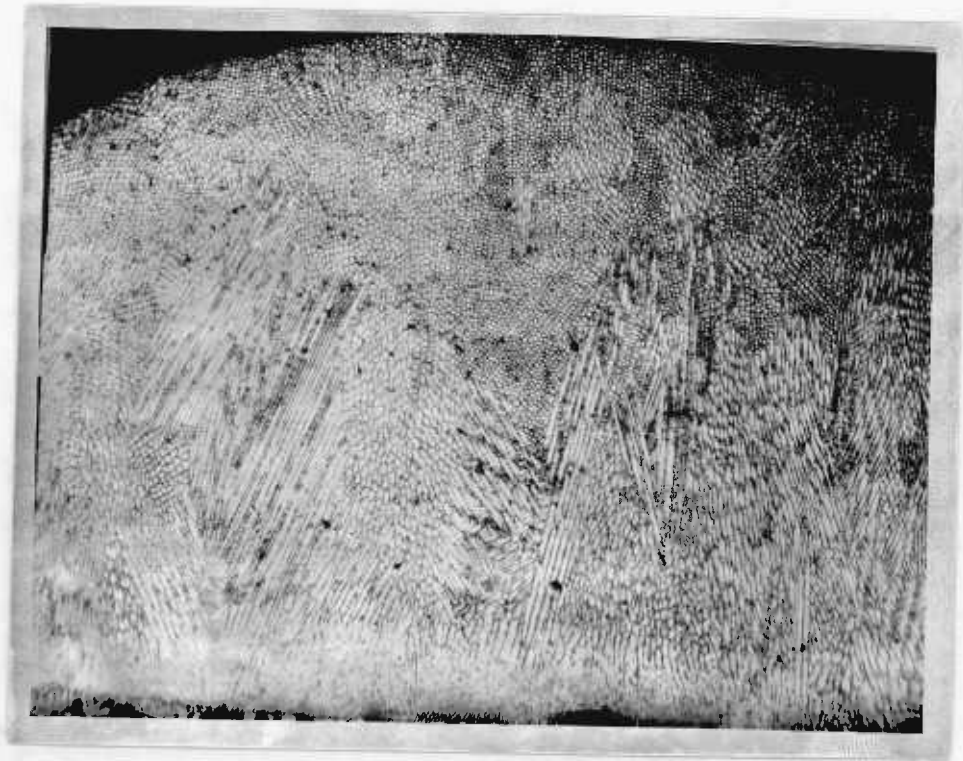
FIG 4.69 MICROSTRUCTURE 316 STAINLESS STEEL CLADDING, SPECIMEN NUMBER S62; POWER=1400 W; BEAM DIAMETER=5.8 MM; SPEED=5 MM/S; POWDER THICKNESS=1.00 MM; ETCHED IN HCl + HNO 3 AND H 2 O SOLUTION, X110.
