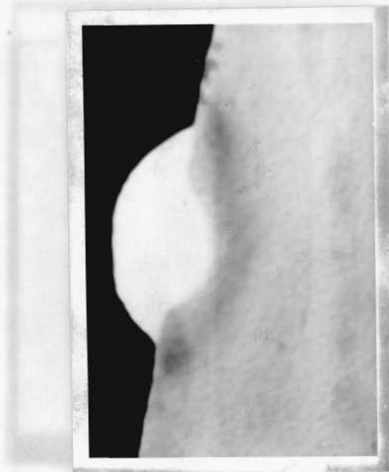
FIG 489 MICROHARDNESS AND MACROGRAPH SECTION VIEW THROUGH SURFACE CLADDING ETCHED 2% NITAL, X21, POWER=1 600 W BEAM DIAMETER = 4.3 MM, SPEED=5 MM/S, POWDER THICKNESS = 1.00 MM.
