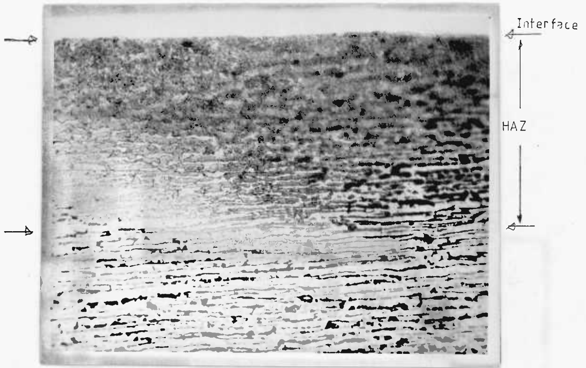
FIG 4.77 HEAT AFFECTED-ZONE IN En 3 STEEL AFTER LASER CLADDING - 316 STAINLESS STEEL, SPECIMEN NUMBER M4; POWER=1 300 W; BEAM DIAMETER=2.29 MM; SPEED=15 MM/S; POWDER THICKNESS=2.00 MM; NO PREHEAT; OVERLAP=1.88 MM; ETCHED IN 2% NITAL; X 110.
