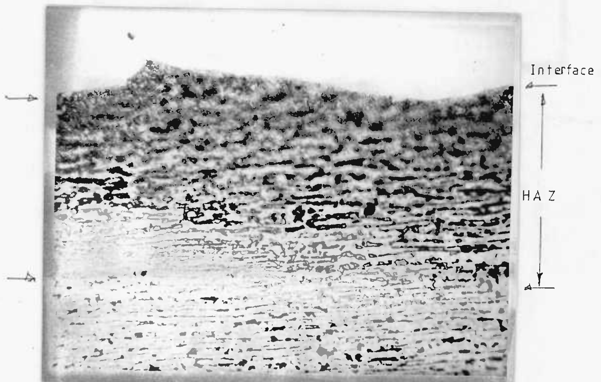
FIG 4.78 HEAT AFFECTED-ZONE IN En 3 STEEL AFTER LASER CLADDING - 316 STAINLESS STEEL, SPECIMEN NUMBER M16; POWER=1 400 W; BEAM DIAMETER=2.29 MM; SPEED=20 MM/S; POWDER THICKNESS=2.00 MM; DEGREE OF PREHEATING=150 °C; OVERLAP=1.5 MM; ETCHED IN 2% NITAL; X 110.
