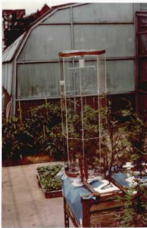
Figure 2.4. Transpiration chamber in use over Cupressus leylandii at South Kensington.
