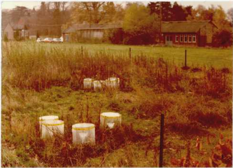
Figure 2.3. Transpiration chambers in use over herbaceous vegetation at Silwood Park.
