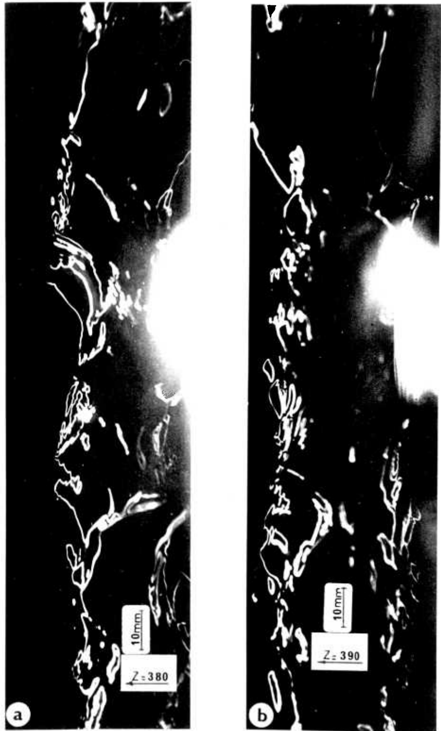
Figure 6.14(a,b): The path of spherical cap shape butane bubbles in water
