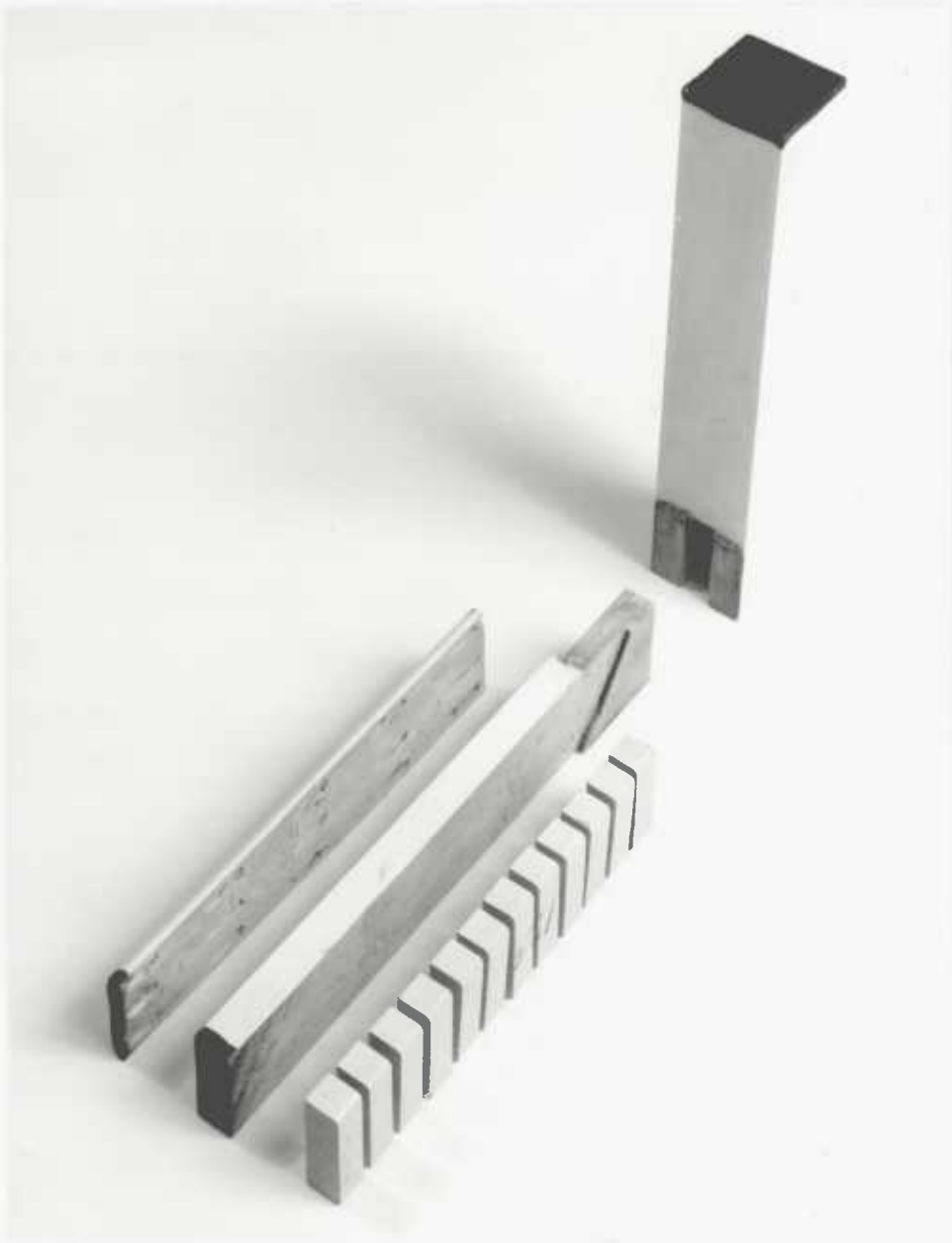
Fig 4.6 Conversion of an L-joint during sampling. (See Fig 4.7)
