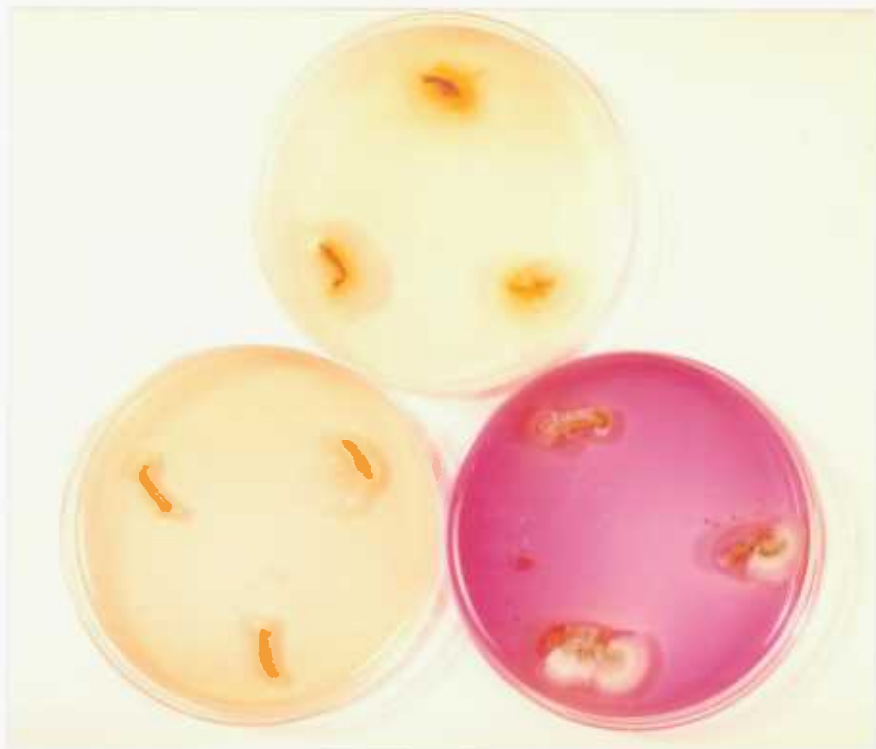
Fig 4.14 Fungal isolations; growth from samples Top two per cent malt agar Left benomyl/malt agar Right starch casein nitrate agar
