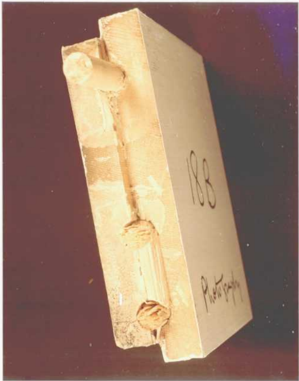
Fig 2.26 Glue squeezed from around the dowels in a joint from a hemlock door. This was one of the best examples of spread of the glue although large areas are still not covered.
