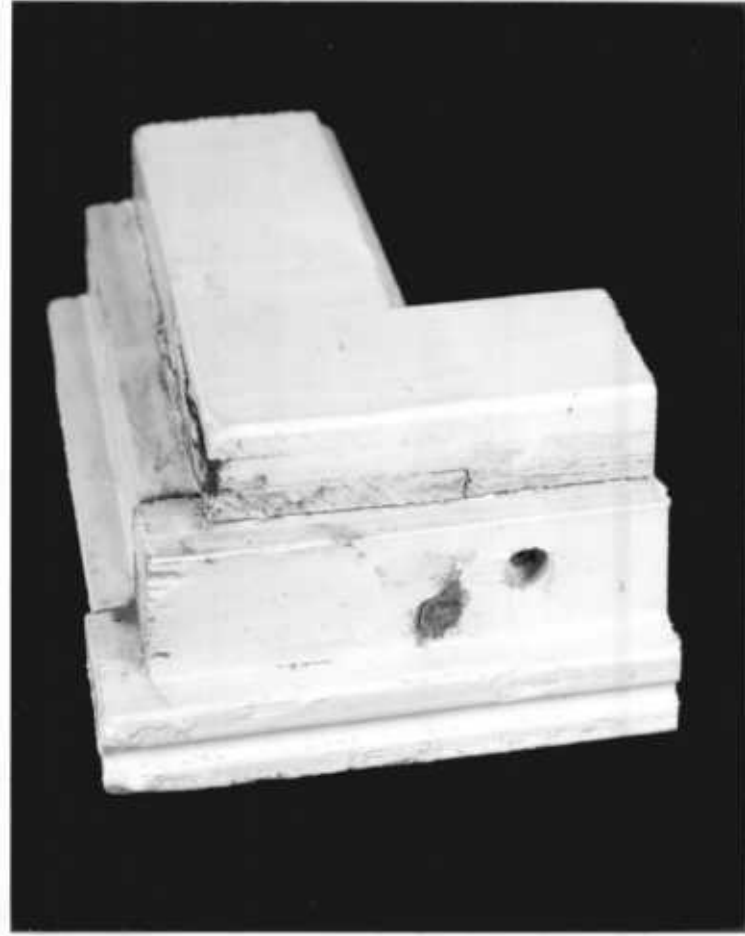
Fig 2.10 Gosport; use of mastic in an attempt to prevent moisture entry. (The horizontal joint (left) and the vertical joint (right) had been drilled out, filled with mastic and the hole closed with a timber plug.)
