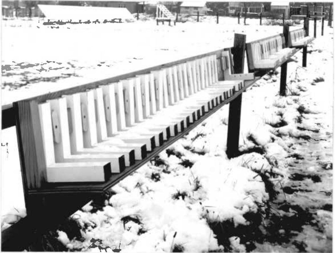
Fig 3.1 L-joints on exposure racks
