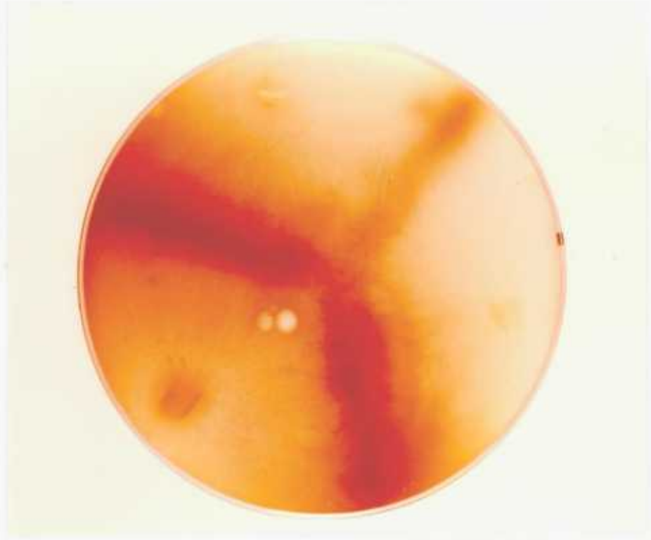
Fig 5.61 Basidiomycete cultures from L-joint No 38. Top b, left a, right c.
