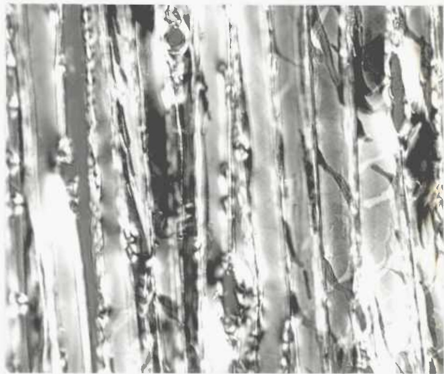
Fig 3.22 Atypical attack (x 275) Above, normal light Below, polarised light
