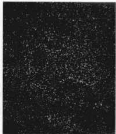
d. X-ray scanning image of (c), showing the distribution of Zr, K \alpha .
