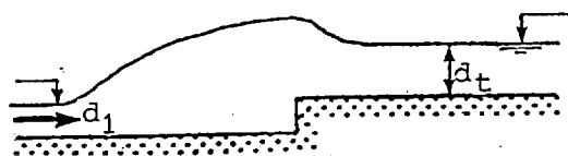
(c) Jump formation at an abrupt rise
