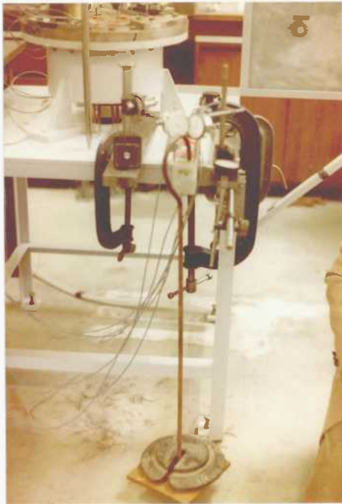
Fig. 5.42. Experiment arrangement of G.R.P. test beam.
