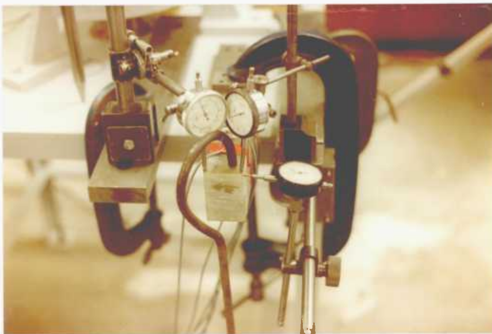
Fig. 5.43. Experiment arrangement of G.R.P. test beam.
