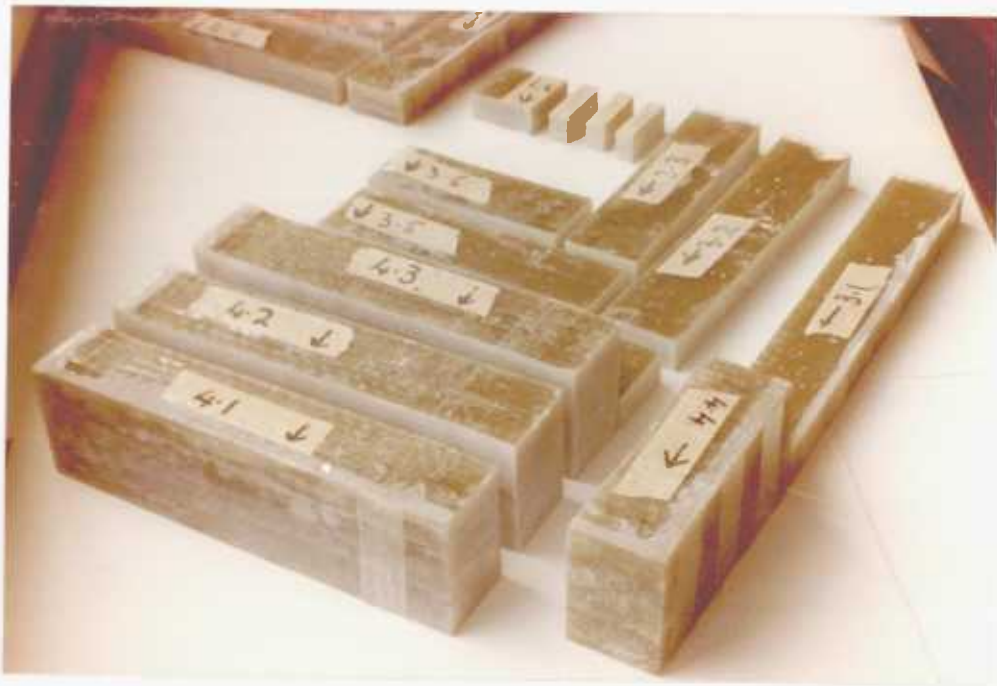
Fig. 5.6b. Composite deep beam specimen
