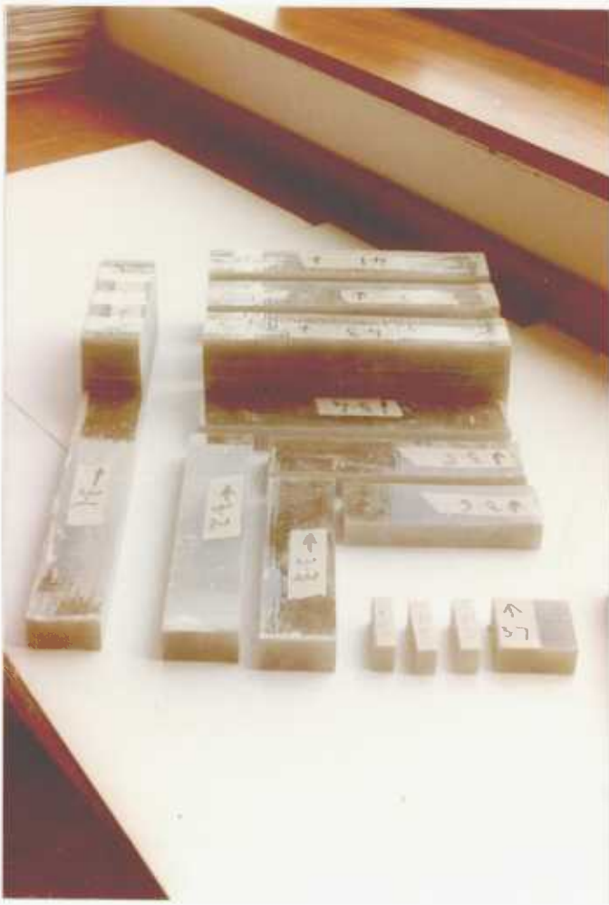
Fig. 5.6a. Composite deep beam specimen
