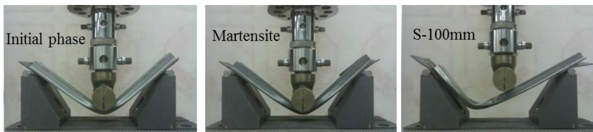
Fig. 8 Failure modes under bending for boron steel parts having different microstructural topographies.
