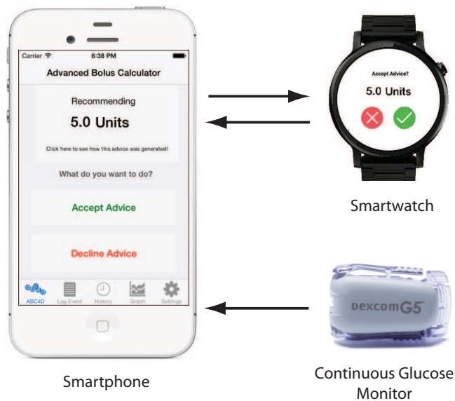
Figure 6.1: Smartwatch version of the ‘Advanced Bolus Calculator for Diabetes’ communicating with the ABC4D patient smartphone platform and synchronising data from a CGM system.
