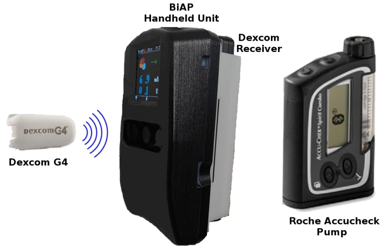
Figure 2.3: Bio-inspired Artificial Pancreas System [11] (centre) communicating with a continuous glucose sensor (Dexcom G4 ® ) and an insulin pump (Roche ACCU-CHECK ® )
