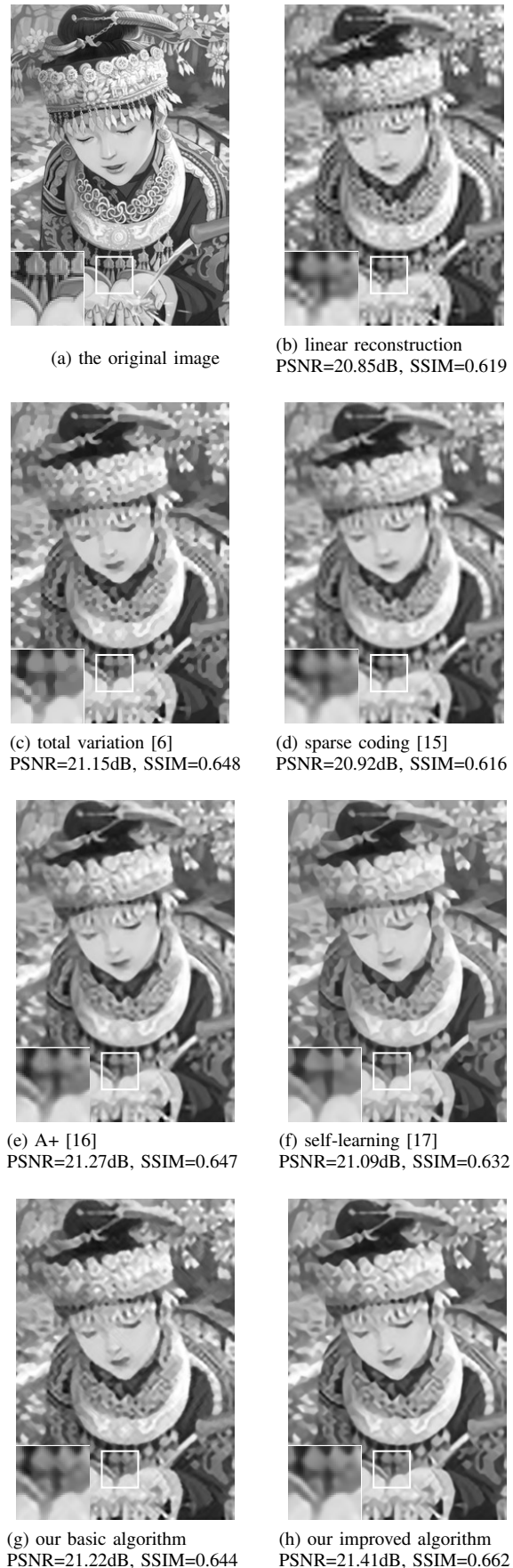
Fig. 17. Upsampling results (factor 4) of Comic by different methods. The downsampling kernel is linear spline.
