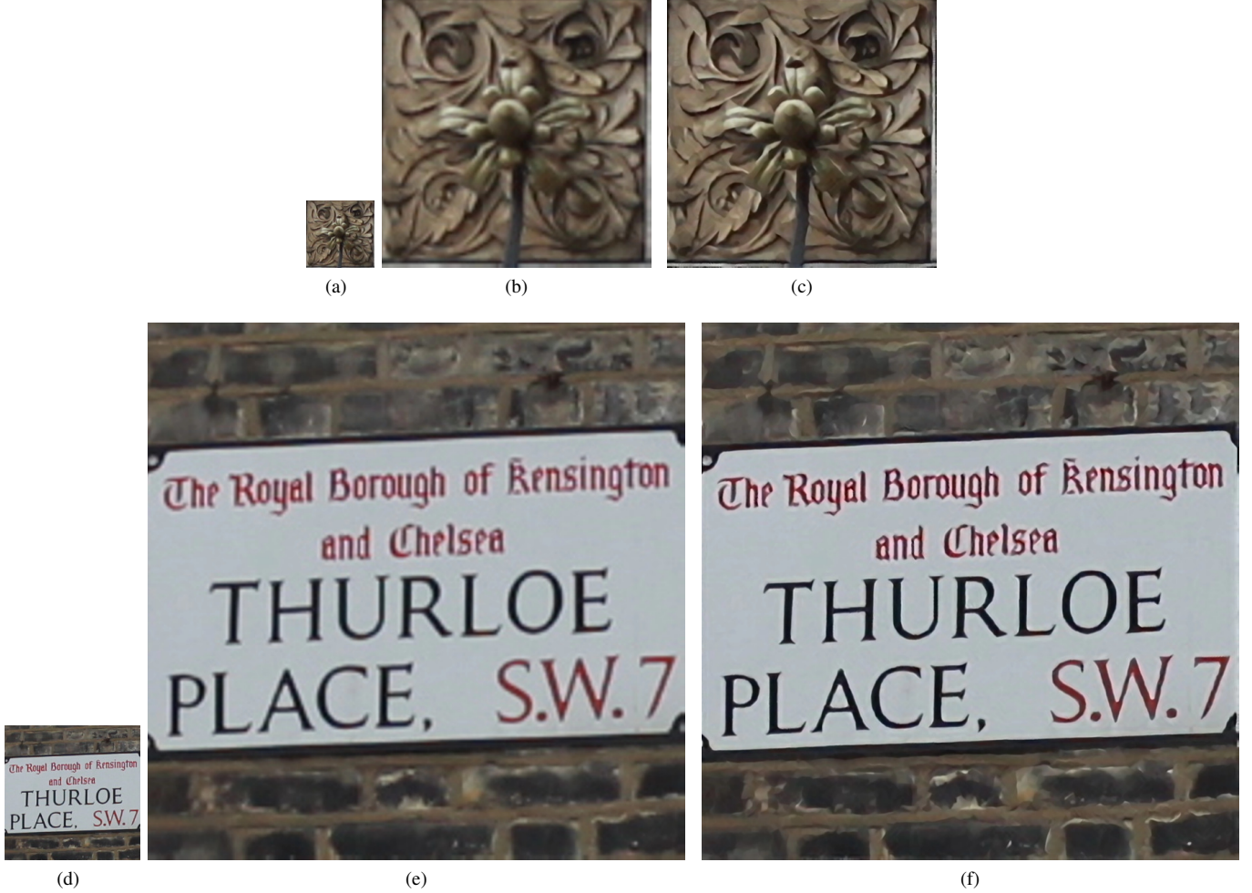
Fig. 18. Upsampling results (factor 4) of images taken with Canon 400D. Our upsampling results are sharper than the bicubic interpolation results. (a)(d) original images. (b)(e) bicubic interpolation. (c)(f) our upsampling results.
