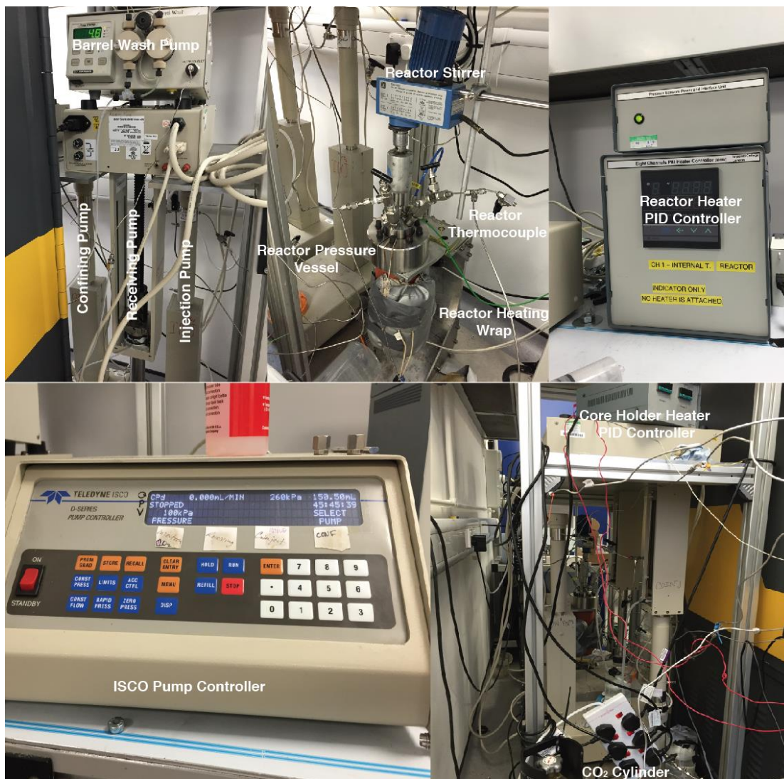
Figure 4.1 Instrumentation outside the \mu -CT consists of three ISCO pumps, a barrel wash pump, a reactor complete with heating and stirring, an ISCO pump controller and two PID heating controllers.
