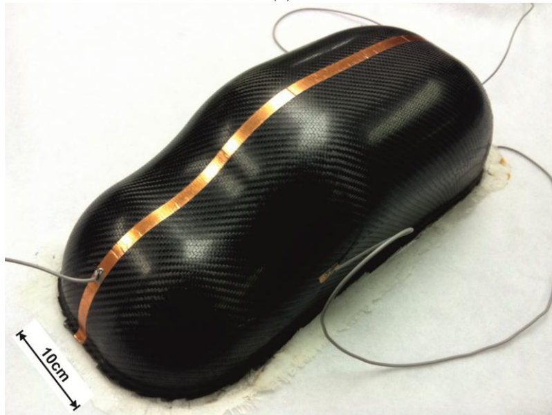
Figure 1 (a) Architecture of the structural supercapacitors and (b) example of a working device.
