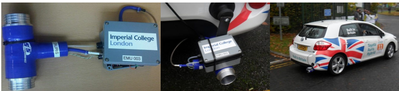
Figure 3.1 – in-house developed Emissions Monitoring Unit (EMU)
