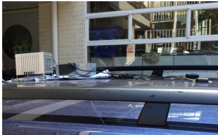
Figure 3.6 – the Hermes trajectory monitoring unit and reference iMar INS installed on the roof of a test vehicle
