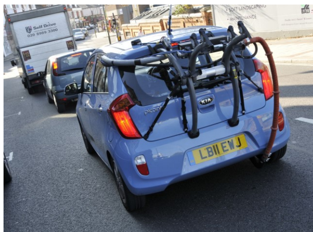
Figure 3.2 – the flow tube connected to a test vehicle during emissions testing (Emissions Analytics, 2015a)
