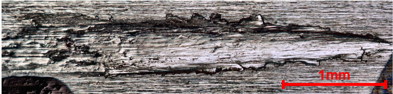
Figure 9: A high dynamic range (HDR) image of the very start of the smearing mark on the lower raceway from Test 2 in Table 2 ( P_{\max} = 3.14 kN, V = 4.53 m/s)
