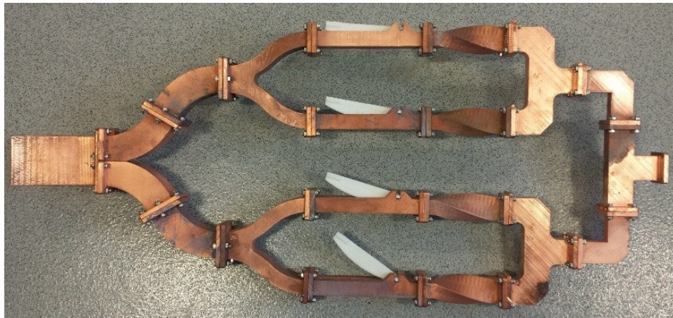
Figure 3.23: Full 3D printed phased array antenna system (including feed splitters, phase shifters and antenna adaptor block).
